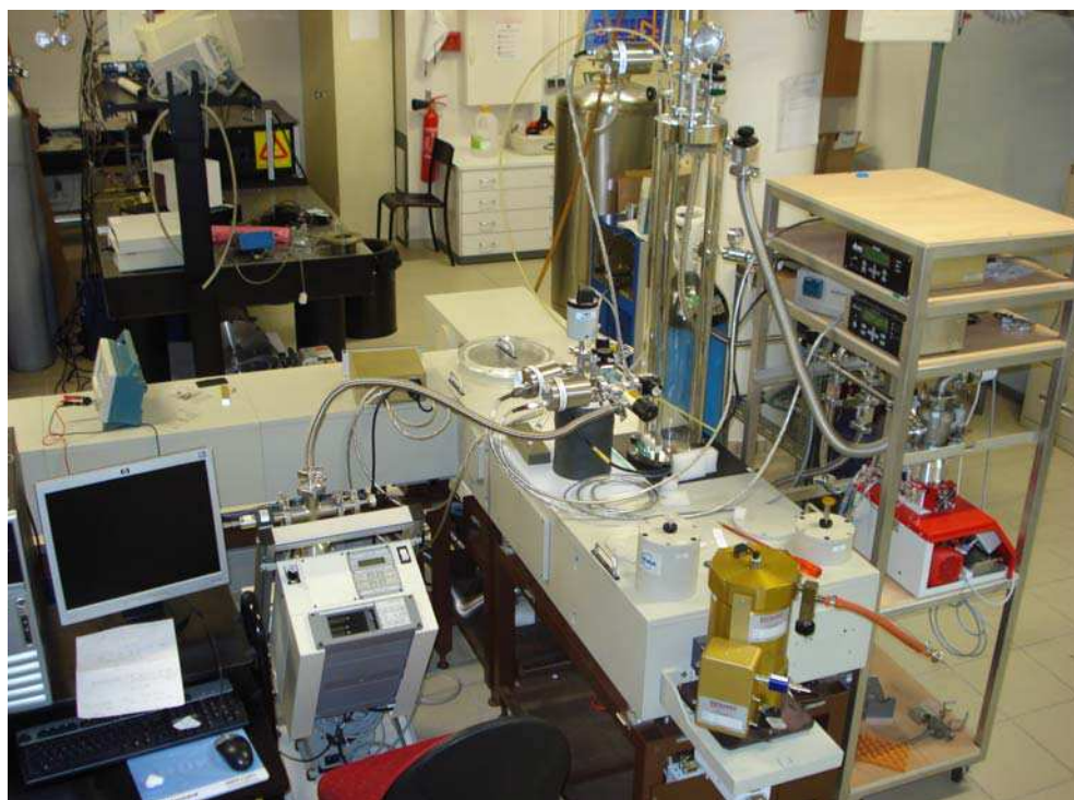
Fig. 3. View of the laboratory showing the Fourier transform spectrometer Bruker IFS125HR, two multiple-reflections Pyrex absorption cells and a gas handling system including a turbomolecular pump. In the back is an optical table with a difference frequency generation (DFG) laser system developed at LPPM in Orsay and LISA in Créteil
