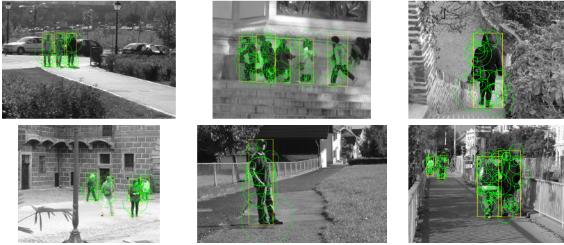
Figure 6.7.: Examples of person height ISM training/testing images. Top: three example training images with detected SURF features within the person bounding box from the INRIA training data set used to train the ISM based person height estimator. Bottom: three example test images from the INRIA test data set used to evaluate the person height estimator.
