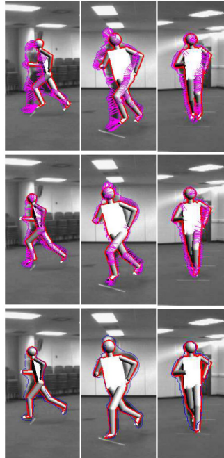
Figure 2.15.: Examples of estimated poses from a publication using person silhouettes (Iterative Closest Points approach).
