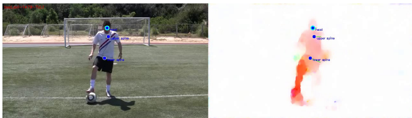
Figure 9.1.: Semi-automatic annotation of 2D poses. Optical flow (here: TV-L1) is used to track three landmarks, annotated for a sparse set of frames by a user. The green lines indicate the direction into which the landmarks move in the next frame based on the optical flow information.
