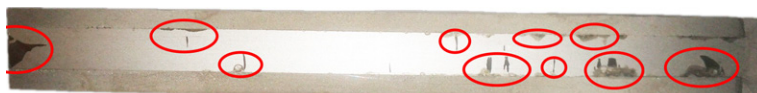
Figure 6.7: A sample without copper plating shows ablating of the silver shunt. The superconductor below is also affected. Some of the damaged regions are marked red.
