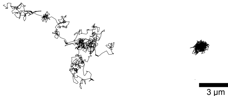
Fig. 3.5 Examples of trajectories of a particle, which freely diffuses through the meshes of the network on the left and a particle, which is trapped by surrounding filaments on the right. In both cases the length of the trajectory is 30 s. The scale bar is the same for both examples.
