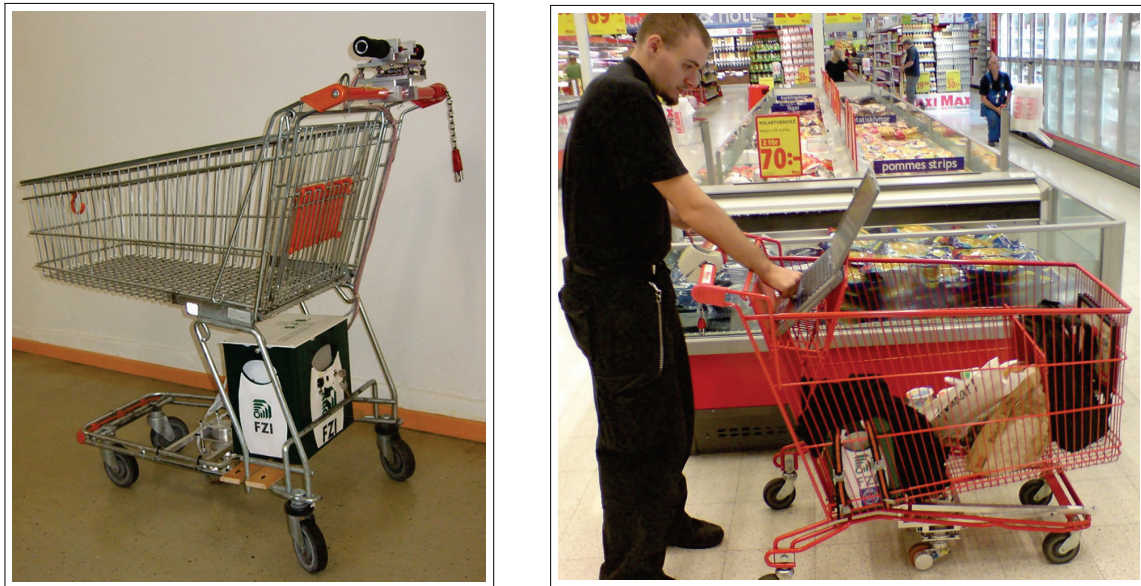
Fig. B.6.: Several versions of ETrolley have been set up: the one shown in Figure B.5, one for tests in the FZI labs including the force sensitive handle (left) and one reduced version for tests in a ICA Maxi supermarket in Stockholm (right, thanks to Helge Hüttenrauch for this opportunity).
