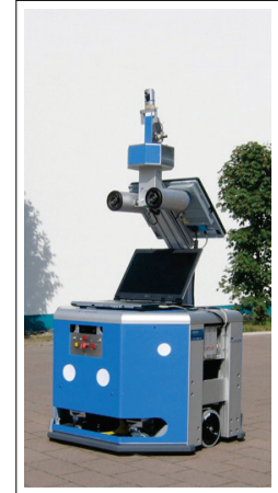
Fig. 2.20.: The autonomous inspection robot MARVIN (image source: [16])
