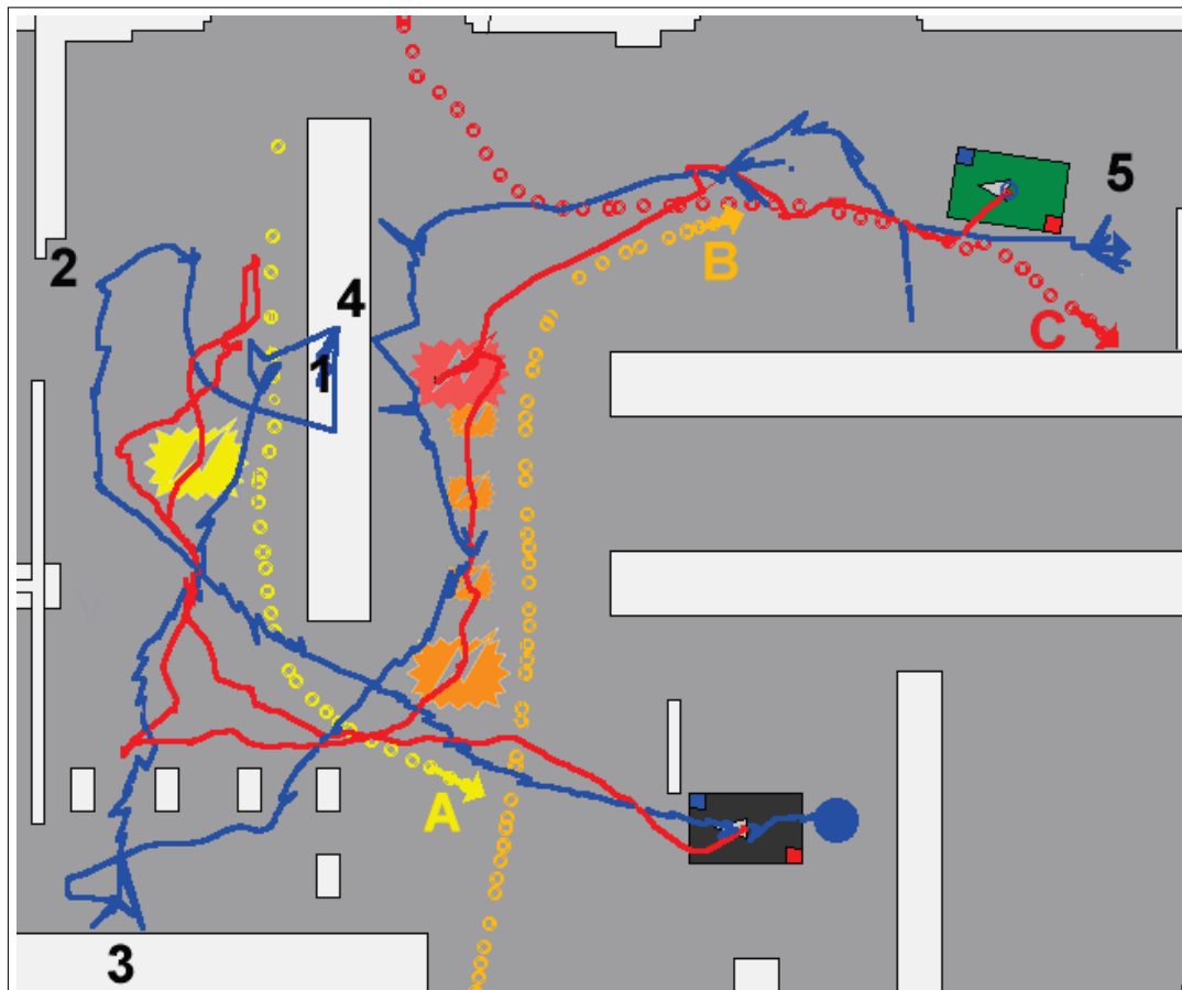
Fig. 5.19.: Final test for avoiding moving objects – a shopping run involving all available functionalities: the user (tracked by the blue line) starts together with the robot (grey rectangle, red line) in the lower right corner. The robot guides the user to the first product (1) while avoiding the moving shopping cart (A) (indicated by the yellow dotted line): the strong bend to the left at the yellow flash symbol. After following the user to the next products (2) and (3), the robot continues to product (4) and avoids the crossing cart (B) (orange dotted line) by slowing down and letting it pass. The robot continues by aligning itself behind the cart (orange flashes). While following to the final product (5) the robot is cut by cart (C) (red dotted line). Again, the robot lets the cart pass (red flash). (Robot's path red, critical areas: flash symbols, the user – who is continuously impairing the robot being another close-by moving obstacle – is tracked by environmental cameras resulting in the chaotic blue line. The bad quality of the user's track comes from continuous occlusions by other objects (shelves, robot, carts, other shoppers, etc).
