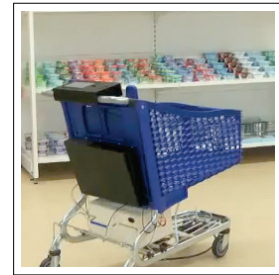
Fig. 2.30.: The Smart Cart by DFKI's Innovative Retail Lab [38]
