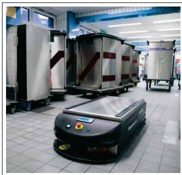
Fig. 1.3.: TransCar automatic guided vehicle (AGV) by Swisslog, operating in hospitals (image source: [157])
