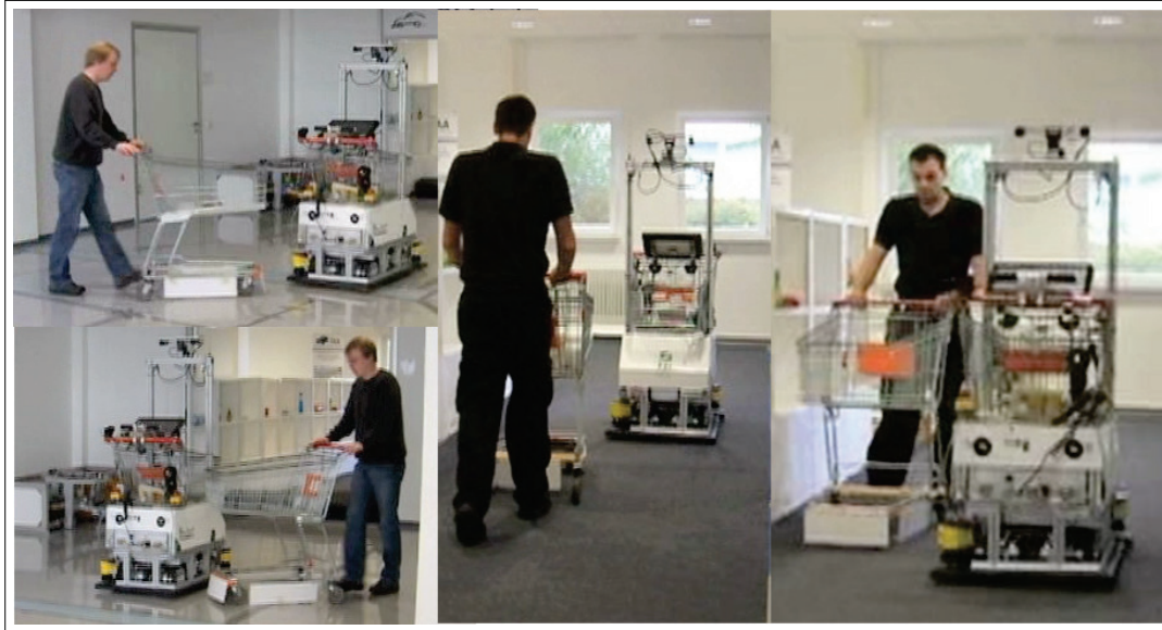
Fig. 5.18.: Photos showing some of the performed tests using a ordinary shopping cart and InBOT 's on-board object tracker. Others have been done using ETrolley to gain precise and robust localization information on the moving object.
