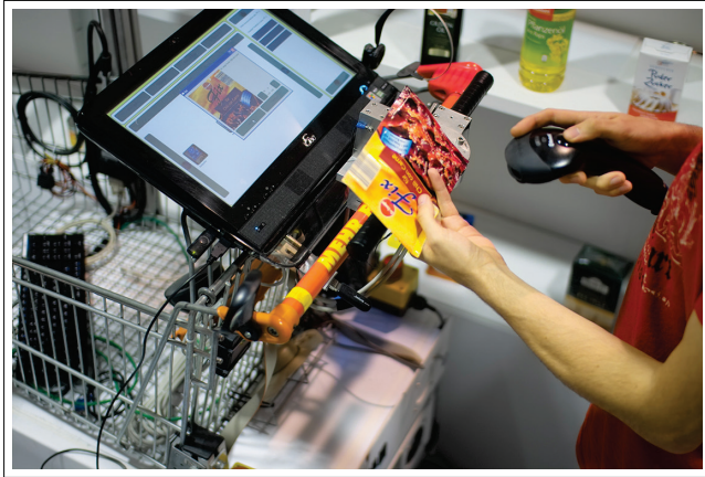
Fig. 6.10.: User scanning a product using the bar code scanner attached to the touch screen user interface
