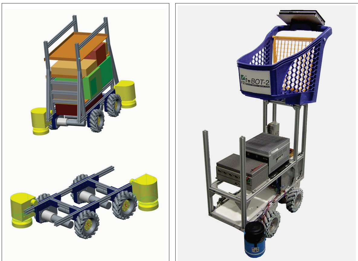
Fig. B.4.: InBOT2 – Left: CAD data. The minimal footprint of the robot is dominated by the size of the two S300 (yellow) and the motors including their gearboxes. The upper levels of the robot's body are designed in a drawer concept, reducing the unused space between the components while providing for easy access to the components. The two major components to be taken into account are the embedded PCs – the green boxes illustrate the bounding boxes including plugs. Right: Current status of the system.
