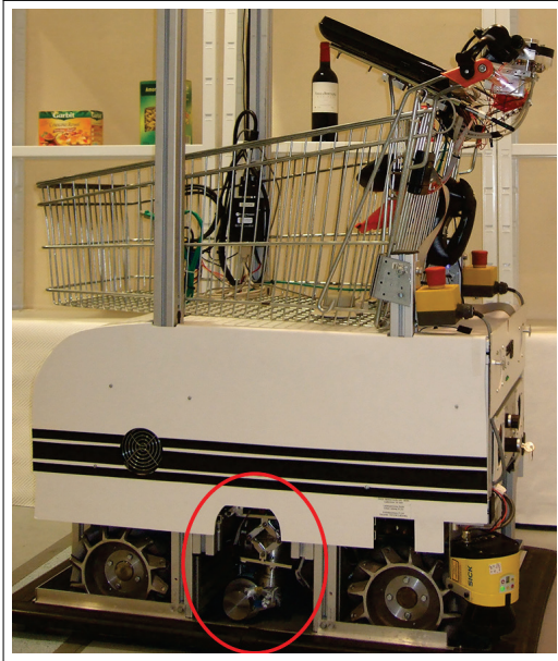
Fig. B.8.: The pair 2D odometry wheels mounted between the front and the back wheels of the mecanum drive track the path of the robot (see Fig. B.14 for a larger picture).
