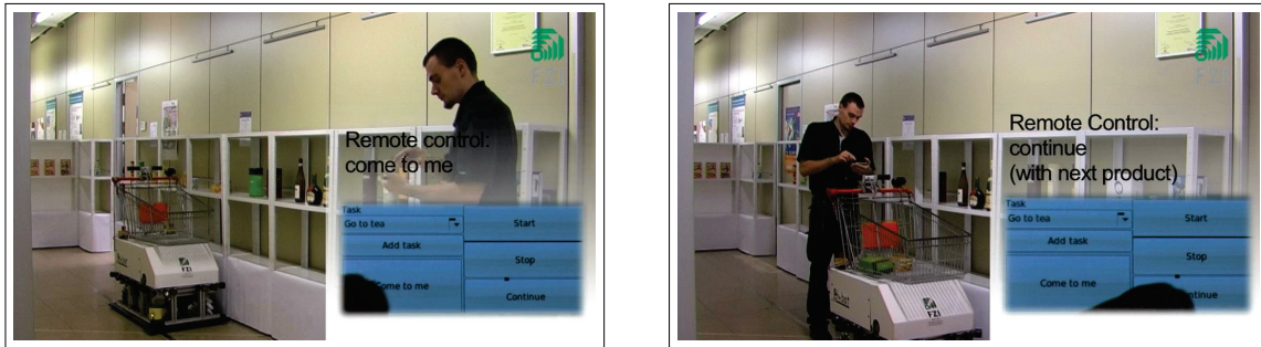
Fig. 6.24.: Commanding InBOT using a smartphone GUI. The smartphone is localized using the WiFi network. The GUI is implemented by the MCAGUI and provides the basic functionalities such as “Stop”, “Come to me”, or “Continue”.
