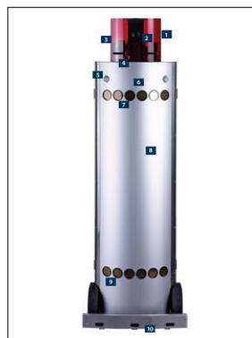
Fig. 2.16.: MOSRO inspection robot with gas detector (image source: [133]) developed by robowatch
