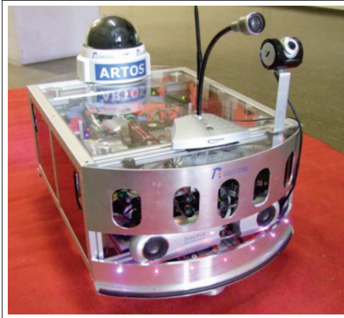
Fig. 2.18.: The autonomous transport robot ARTOS (image source: [109])
