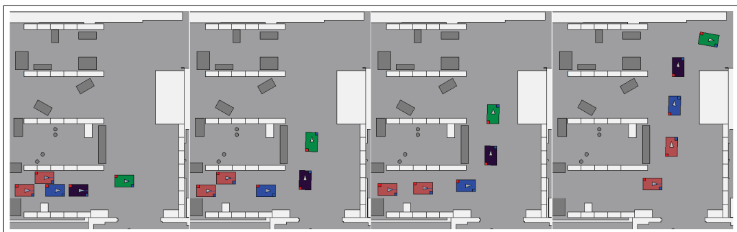
Fig. 7.5.: Forming a virtual train: 5 robots are starting tightly packed with the order to build a virtual train. As they start moving they each wait for their preceding robot to gain a defined distance before starting themselves.
