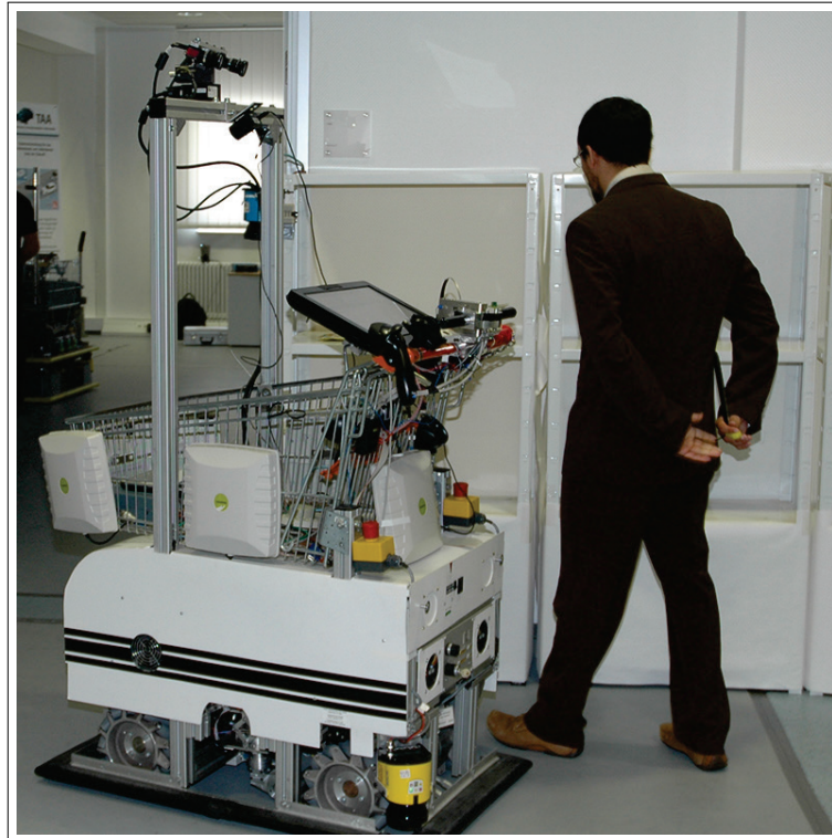
Fig. C.5.: InBOT is following a user who is carrying an RFID tag in his hands by means of RFID localization and color templates of skin and clothes. The white boxes mounted on the basket house the RFID antennas.
