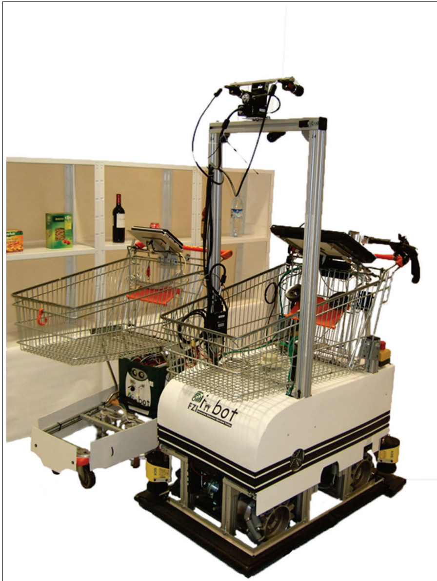
Fig. 1.11.: The shopping robot InBOT and the passive shopping assistant ETrolley
