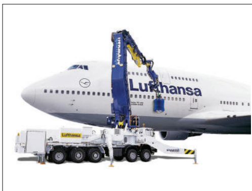
Fig. 2.15.: Airplane cleaning robot Skywash by Putzmeister (image source: [126])
