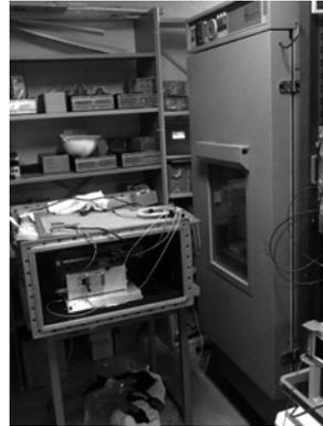
(b) Open VSA shielding box set up next to the temp. controlled chamber.
