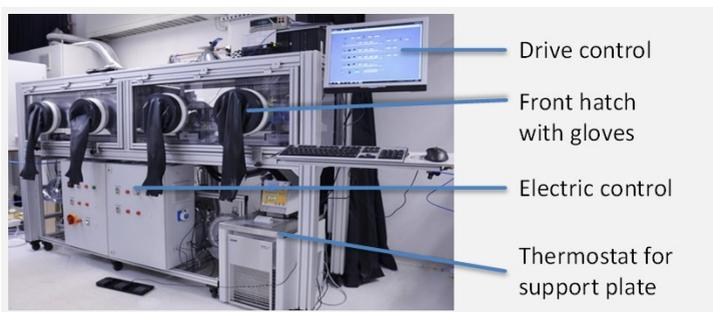
*Figure 2.1: Photograph of the encapsulated coating chamber of the batch-coating and drying set-up.*
