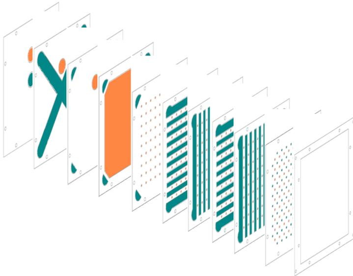
*Figure 9.16: Exploded assembly drawing of the ARN-drier. Inlet and outlet air channels are highlighted by orange and green color, respectively.*
