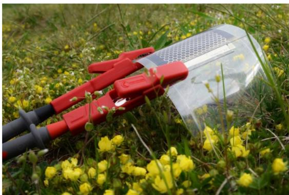
*Figure 7.6: Photograph of a stack of five liquid phase processed functional films for an inverted solar cells. The first four layers were slot-die coated on the pilot coating line.*
