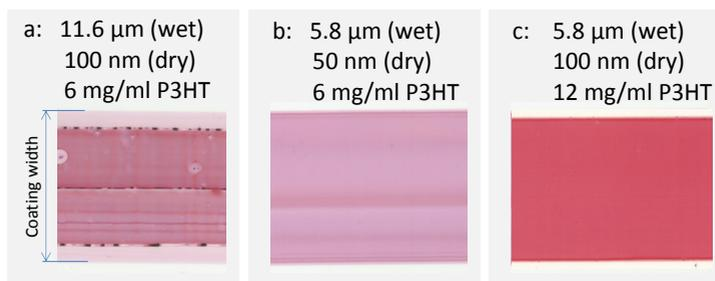
Figure 6.9: Scans of two P3HT-P200:PCBM films slot-die coated and dried under identical conditions (CB:CF = 1:1) but different wet film thickness (a, b) and different solid content (c). The polymer to fullerene ratio was kept constant (1.25).
