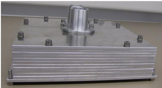
*Figure 9.15: Photo of the compact array of round nozzles.*
