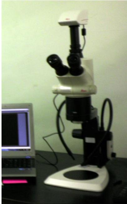
Figure 1.2: Binocular microscope S6 D Leica with magnification of 6.3x - 40x supported by digital camera for sorting and documentation of the samples.
