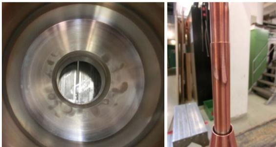
*Surface damages observed on of the anode (left) and coaxial insert (right) created due to the activity of trapped electrons.*
