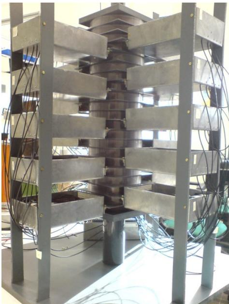
20-stage modular trigger generator during assembly.
