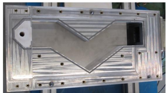
View of the applicator interior. On the left side there is the one of the cavities. On the right side there is one branch of the power divider.
