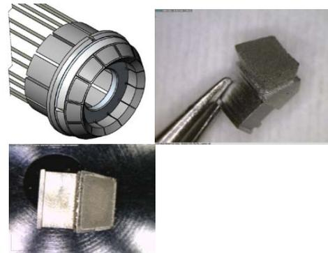
Design drawing of the segmented emitter (top left), manufactured segment (top middle and bottom right).
