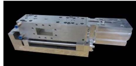
*CAD drawing and fabricated microwave applicator for pultrusion of carbon fiber composites*
