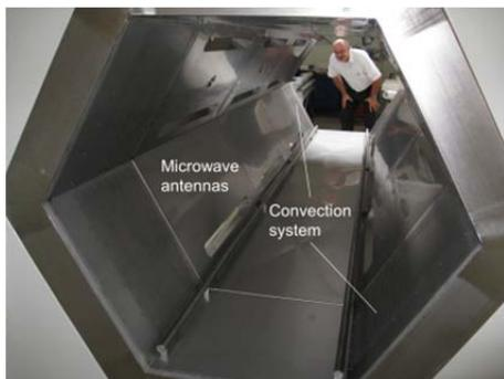
Microwave chamber of the new hybrid HEPHAISTOS prototype
