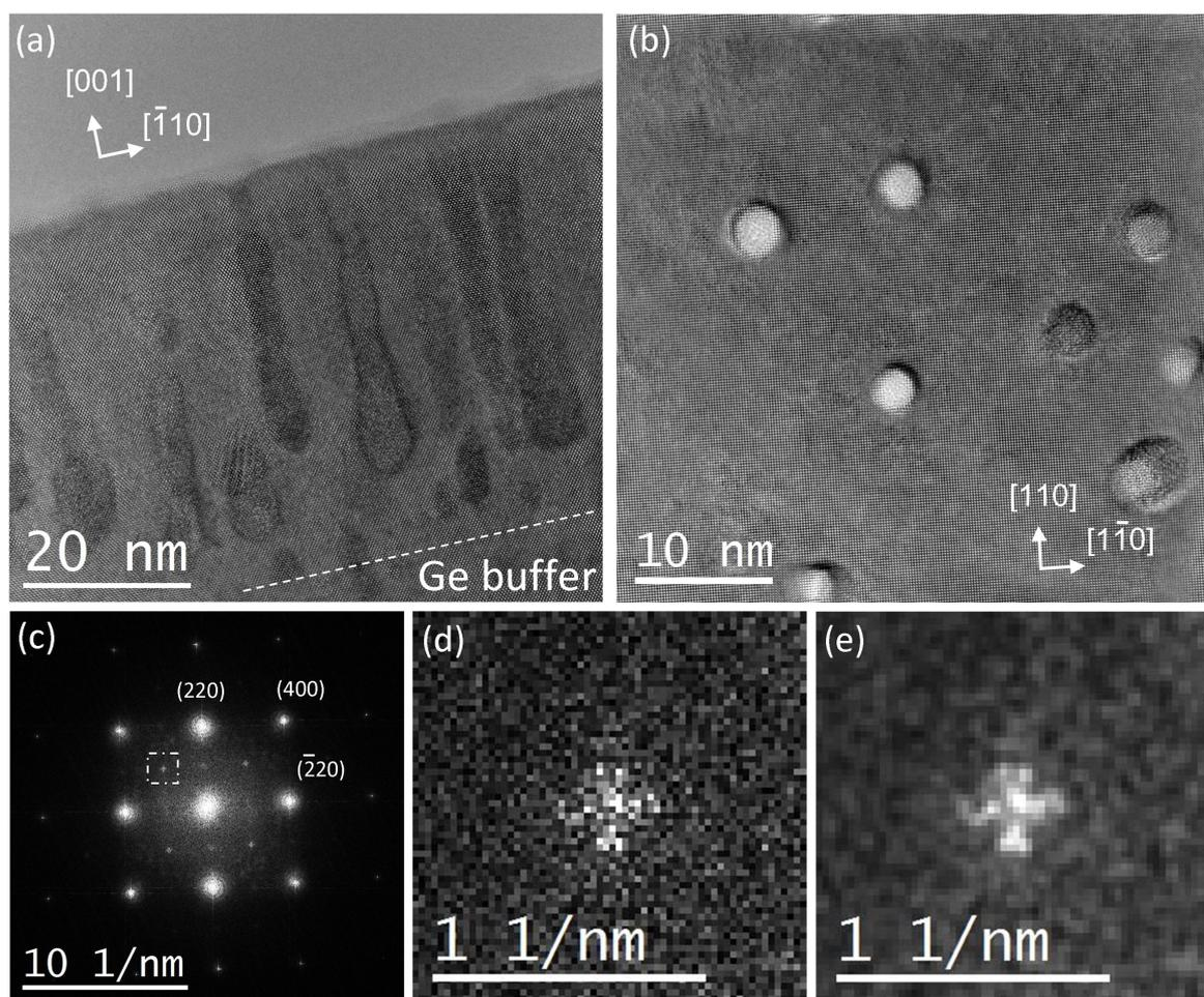
**Figure 5.24.:** (a-b) HRTEM images of the S2 sample in the [110]- and the [001]-zone axis. (c) Power spectrum of the whole image in (b). (d) Zoom on the {020} reflections as indicated by the dashed square in (c). (e) Smoothed image of (d).
