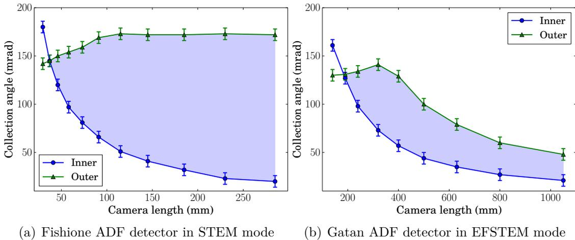
**Figure 2.17.:** Dependence of the collection angles of ADF detectors on the camera length. The fill area represents the scattering angles collected by the detectors. The ADF Fishione and ADF Gatan detector are respectively used as a HAADF detector in STEM mode and EFSTEM mode.
