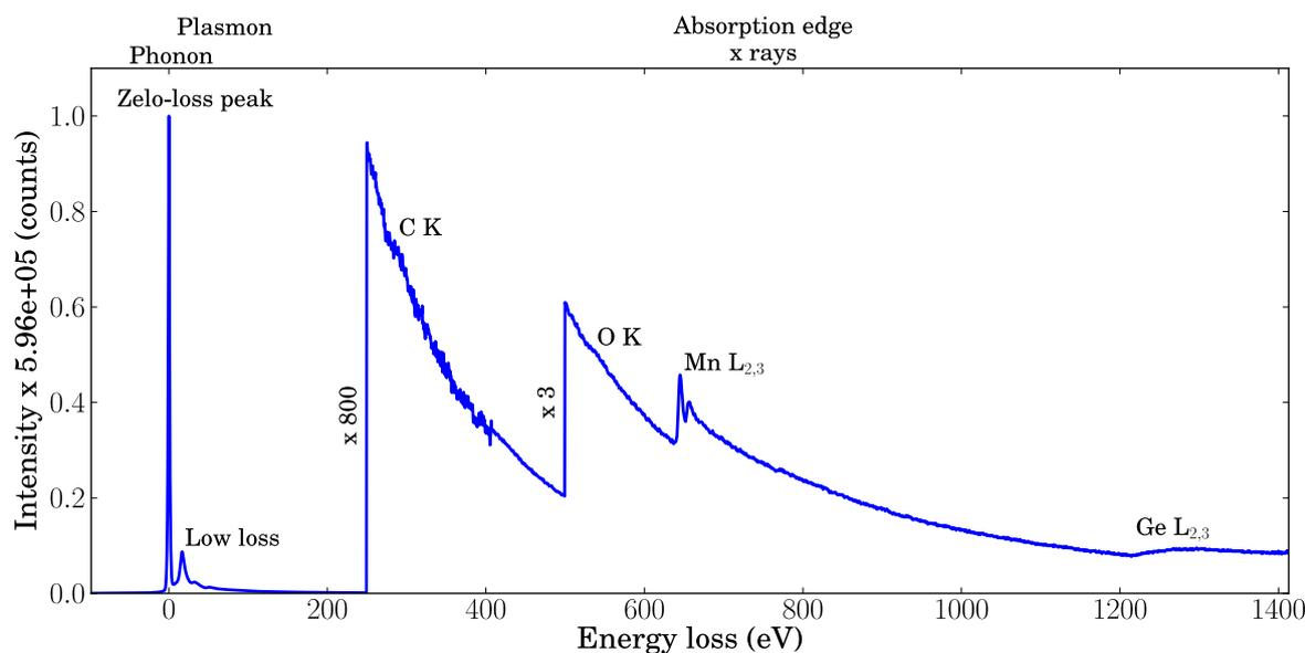
**Figure 2.20.:** Typical EELS spectrum of a GeMn specimen acquired in dual-EELS mode exhibiting the high dynamic range from the zero-loss peak to the core-loss edge of Ge at 1217 eV. The SNR of the carbon edge is poor as it is acquired on the same spectrum than the zero-loss peak. The core-loss spectrum acquired for longer exposure time between 350 eV and 1350 eV has a much better SNR.
