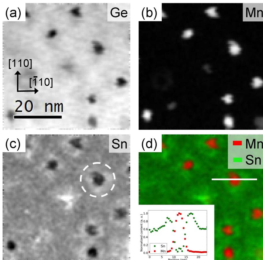
**Figure 5.27.:** Plane-view composition analysis obtained by STEM-EELS measurements of S2 sample: EELS maps of (a) Ge  $L_{2,3}$ , (b) Mn  $L_{2,3}$ , (c) Sn  $M_{4,5}$ . (d) Mn (red) versus Sn (green) composite image. An elemental profile of Mn and Sn across a GeMn nanocolumn and the GeSn matrix at the position marked by a white line in (d) is shown in the inset of (d).
