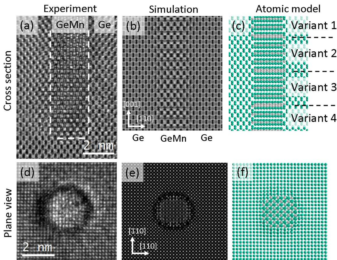
**Figure 5.16.:** Comparison of experimental and simulated HRTEM image of a GeMn NC. (a) Cross-section and (c) plane view experimental HRTEM image. (b, d) Corresponding HRTEM image simulation with a  $\alpha$ -phase in the NC.
