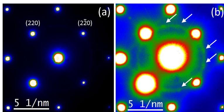
**Figure 5.13.:** SAED pattern of  $\text{Ge}_{0.9}\text{Mn}_{0.1}$  layers grown at temperature of  $130\text{ }^\circ\text{C}$ . The same pattern is displayed on different intensity scale: (a) the whole intensity range (0 to 65535), whereas in (b) the intensity is saturated at 6110.
