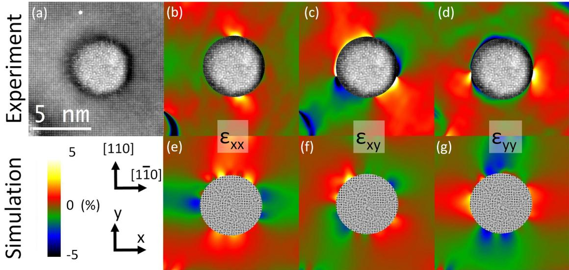
**Figure 5.17.:** GPA around an amorphous NC. (a) HRTEM image of an amorphous NC. (b, c, d) experimental  $\varepsilon_{xx}$ ,  $\varepsilon_{yy}$  and  $\varepsilon_{xy}$  strain map obtained from the HRTEM image shown in (a). (e, f, g) Simulated  $\varepsilon_{xx}$ ,  $\varepsilon_{yy}$  and  $\varepsilon_{xy}$  strain map.
