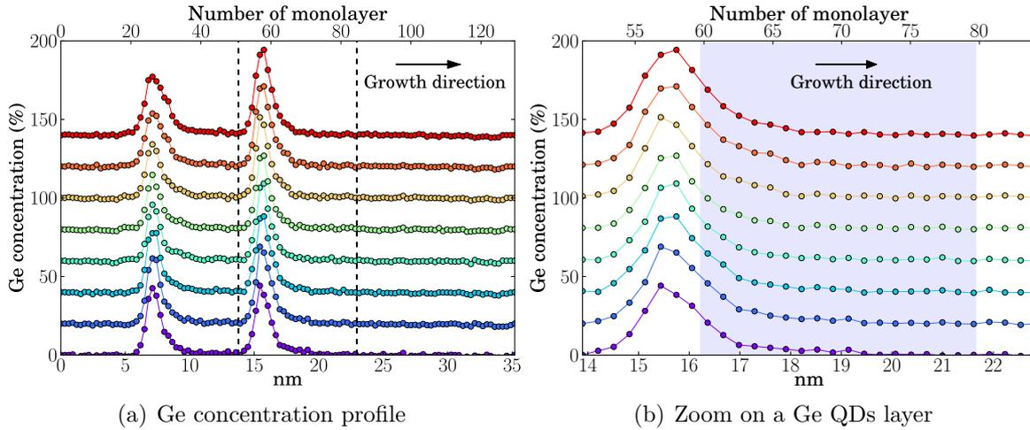
**Figure 4.22.:** (a) Ge concentration profiles across two layer of 4 ML Ge grown on Si(001) substrate obtained by EELS measurements. (b) Zoomed area taken in the region delimited by the dashed lines in (a). The blue filled square indicates the experimental data used for the fit. For clarity, the Ge concentration profile are separated by an offset of 20 %.
