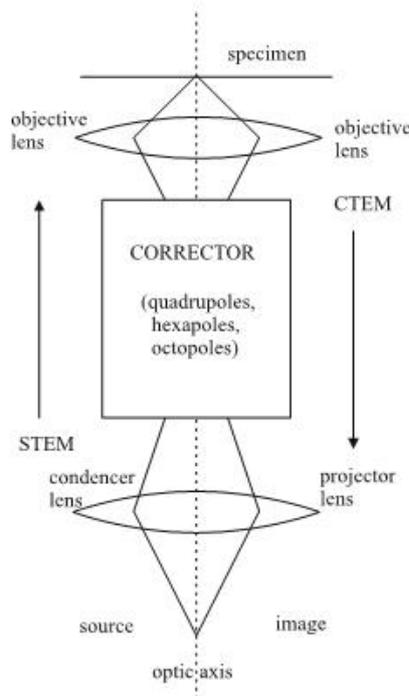
**Figure 2.5.:** Placement of the corrector in the column for STEM and CTEM mode. The labels on the left and right side correspond to the STEM and TEM configurations, respectively. The corrector introduces a negative  $C_3$  to counterbalance the positive  $C_3$  of the objective lens. Taken from [Kirk 10].
