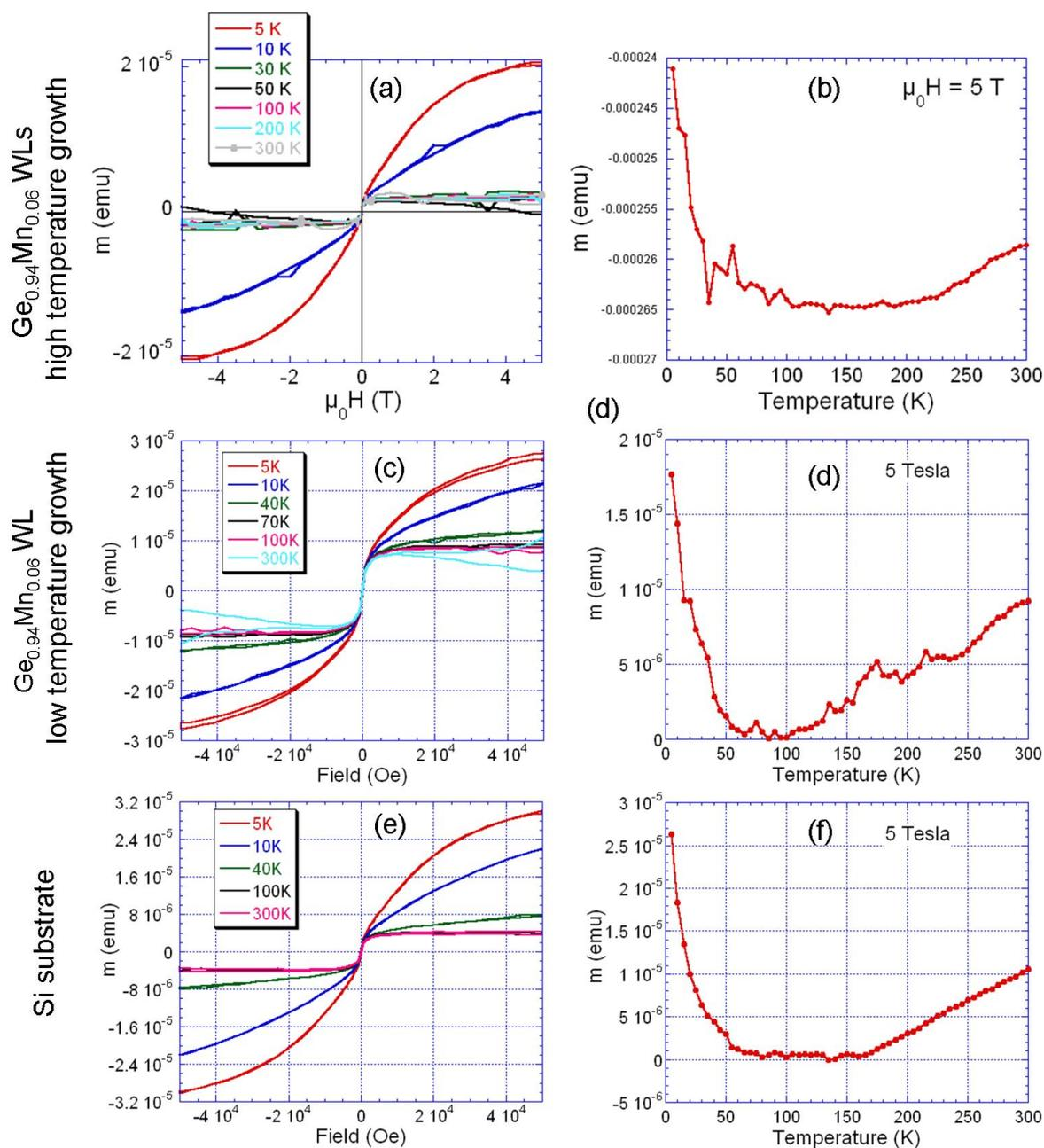
**Figure 4.32.:** Magnetic investigations using SQUID of different specimen: (a-b)  $\text{Ge}_{0.94}\text{Mn}_{0.06}$  WLS (4 ML) grown at high temperature (380 °C), (c-d)  $\text{Ge}_{0.94}\text{Mn}_{0.06}$  WLS (4 ML) grown at low temperature (220 °C) and (e-f) Si substrate. (a,c,e) Magnetization loop measured at different temperature. (b,d,f) Temperature dependence of the saturation magnetization.
