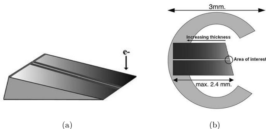
**Figure 2.25.:** Schematic view of the prepared sample in cross-section. (a) Shape of the sample showing increasing thickness of the wedge, the glue line and the layer of interest. (b) Sample glue on a grid with two thin area of interest at the edge of the wedge. Scheme taken from [Ayac 10].
