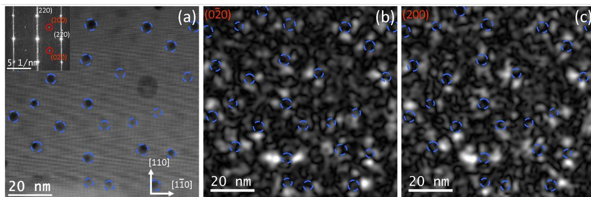
**Figure 5.26.:** (a) HAADF-HRSTEM image of S2 samples. In the inset of (a) shows the power spectrum of the HAADF images in (a). (b, c) Amplitude of the Fourier component corresponding to the  $(0\bar{2}0)$  and  $(200)$  forbidden Bragg reflections, which are marked by red fill circles in the inset of (a). The blue dashed circle indicated the position of the NCs.
