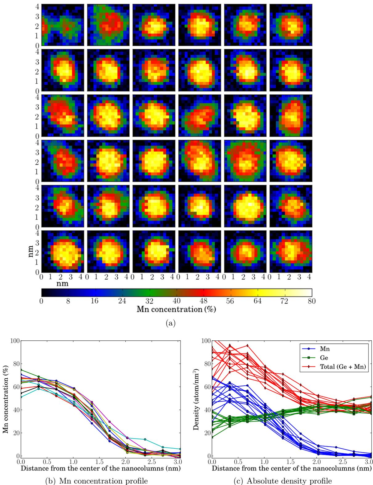
**Figure 5.5.:** (a) Set of NCs used for the statistical analysis of Mn composition in NCs. Radial profile of (b) Mn relative concentration and (c) Mn, Ge and total density. The sub-image in (a) come from the Mn concentration map shown in Fig. 5.4(d) and are displayed on the same color scale. The radial profiles in (b-c) go from the fitted center the NCs to the Ge substrate.
