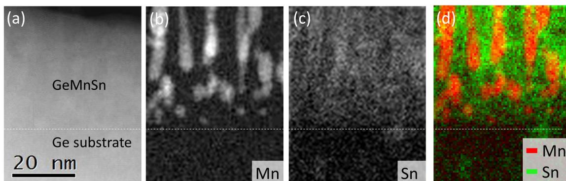
**Figure 5.28.:** Cross-section composition analysis obtained by STEM-EELS measurements of S2 sample: (a) HAADF images recorded simultaneously. (b) Mn  $L_{2,3}$  and (c) Sn  $M_{4,5}$  map. (d) Mn (red) versus Sn (green) composite image.
