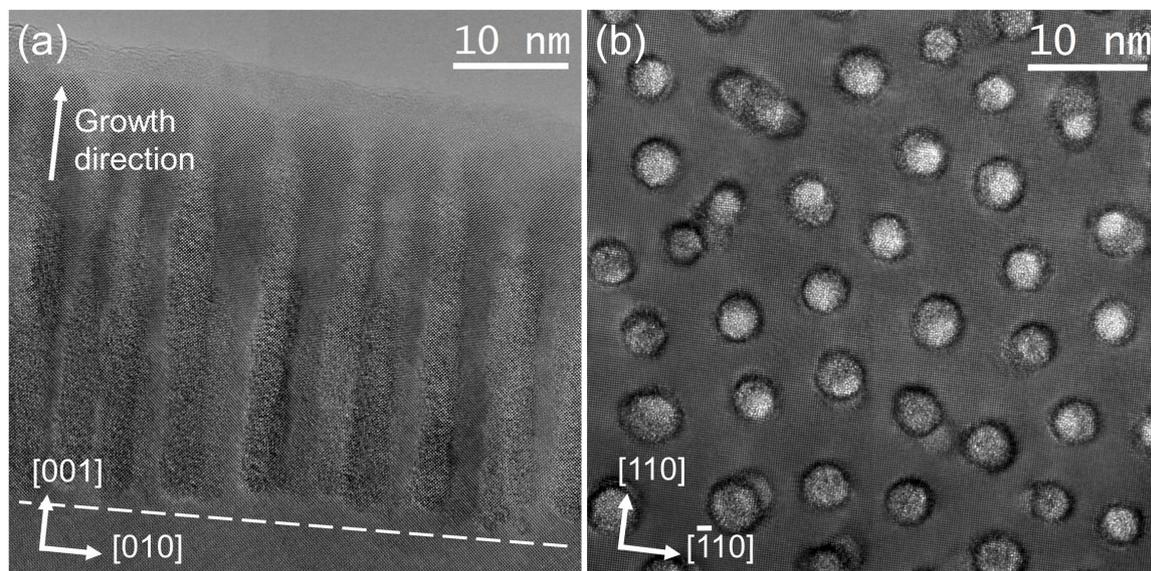
**Figure 5.2.:** 200 kV aberration corrected HRTEM images of a  $\text{Ge}_{0.9}\text{Mn}_{0.1}$  showing nanocolumns (a) in [100]-zone axis (cross-section view) and (b) in [001]-zone axis (plane view). The dashed in (a) indicate the interface between the Ge(001) buffer and the GeMn layer.
