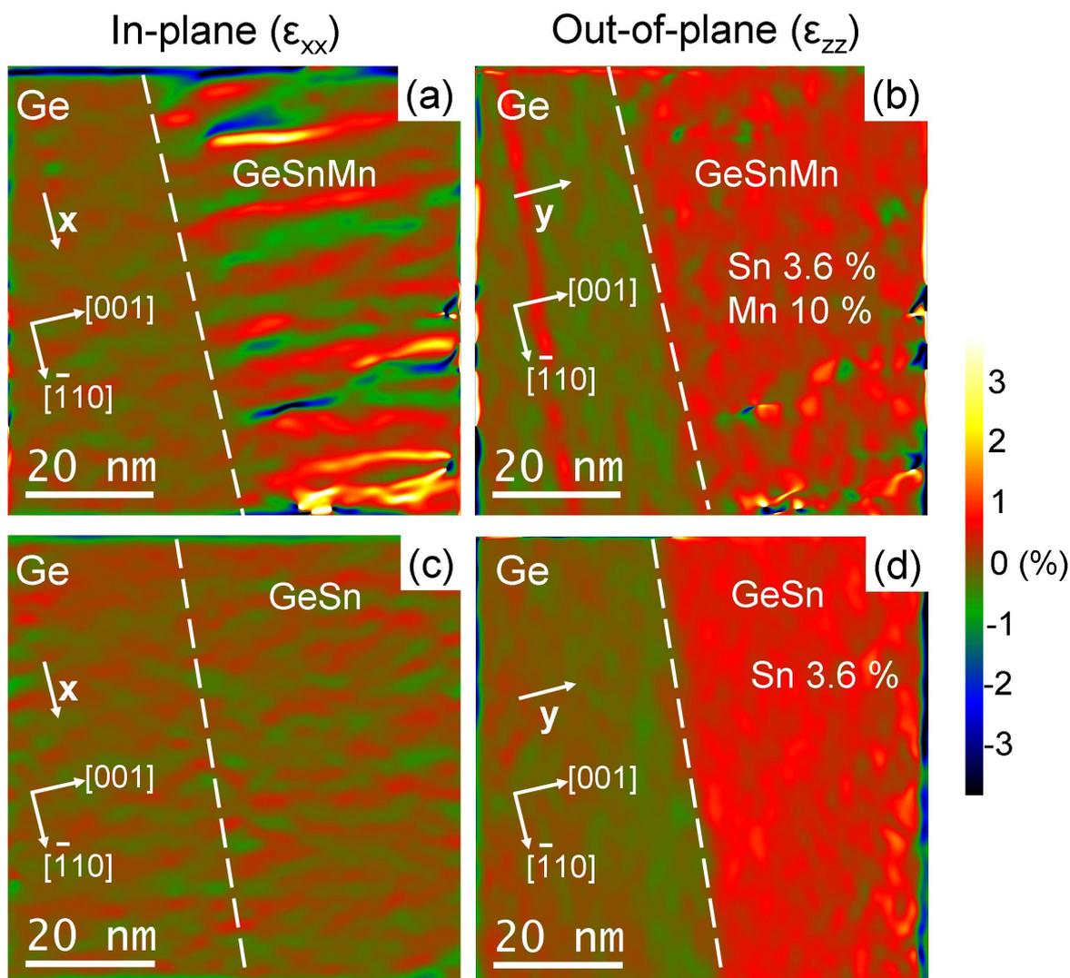
**Figure 5.29.:** GPA performed on HRTEM images of a  $\text{Ge}_{0.84}\text{Sn}_{0.06}\text{Mn}_{0.10}$  film in  $[110]$ -zone axis (a-b) and a  $\text{Ge}_{0.94}\text{Sn}_{0.06}$  film (c-d), both with 6 % Sn. (a,c) In-plane ( $\varepsilon_{xx}$ ) and (b,d) out-of-plane ( $\varepsilon_{zz}$ ) strain maps.
