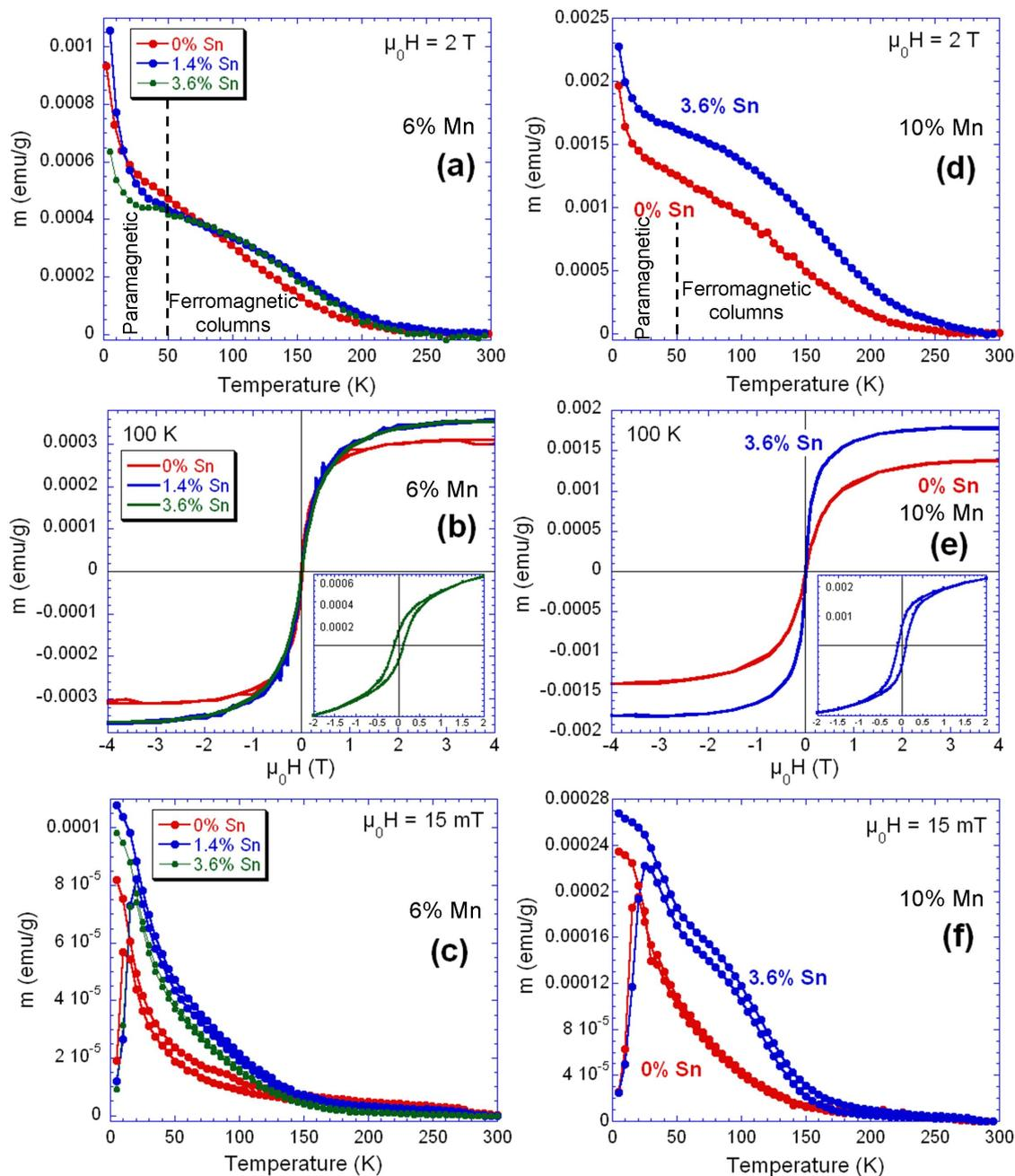
**Figure 5.31.:** SQUID results of GeSnMn film with 6 % Mn (a-c) and 10 % Mn (d-f). (a,d) Temperature dependence of the saturation magnetization. (b,e) Magnetization loops at 100 K, after subtracting the diamagnetic contribution from the substrate. (c,f) Zero field cooled-field cooled measurements carried out at 15 mT.
