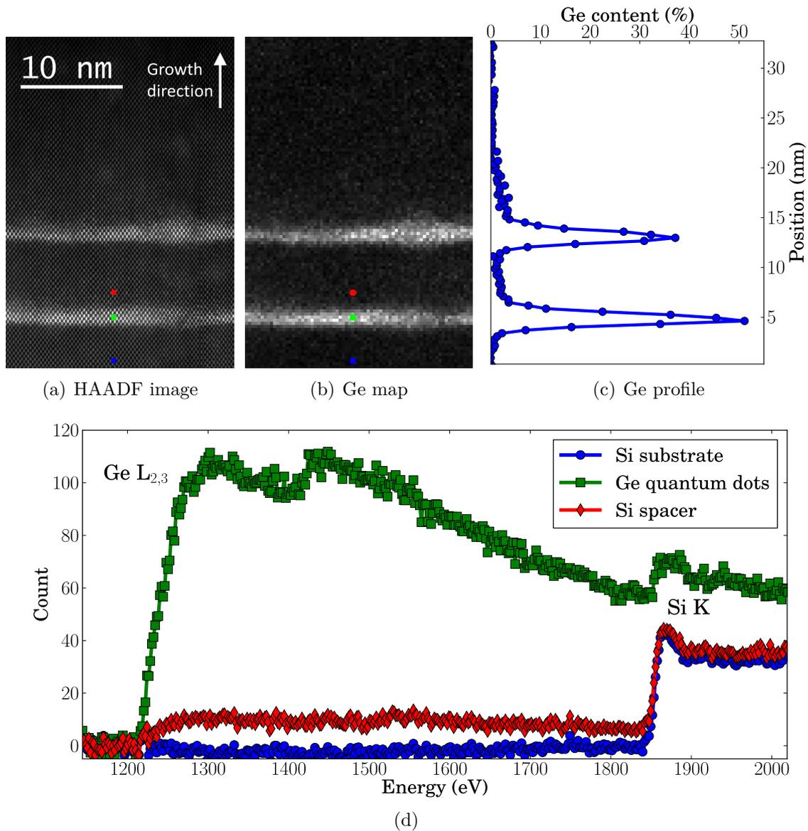
**Figure 4.14.:** (a) HAADF image acquired simultaneously with the EELS SI. (b) Ge map obtained by EELS. (c) Ge concentration profile across the Ge quantum dots averaged over 20 pixels. (d) Background subtracted EELS spectra extracted of unique pixel at different position of the EELS SI as indicated the square of the corresponding color in (a) and (b). For EELS acquisition the probe current was 85 pA and PCA denoising was performed with three components.
