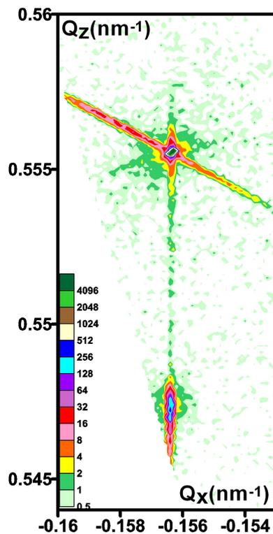
Figure 5.21.: X-ray map around the  $[\bar{1}\bar{1}5]$  Bragg peak of a 250 nm thick  $\text{Ge}_{0.94}\text{Sn}_{0.06}$  layer grown on Ge(001).
