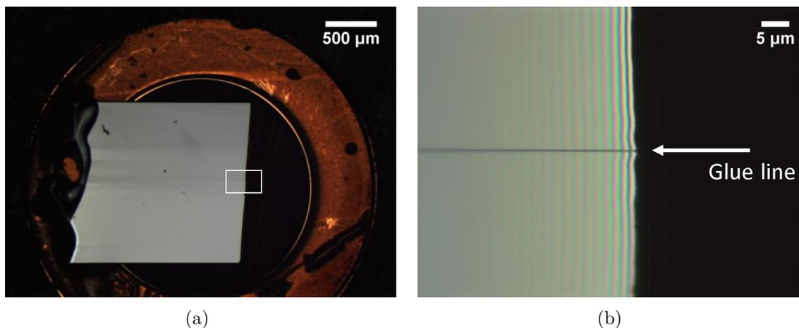
**Figure 2.26.:** Light microscopy images of (a) Si-based  $2^\circ$  wedge sample glued on Cu grid and (b) zoom on the area of interest marked by a white square in (a). Two pieces of sample are glued together face to face and are separated by a glue line (dark line in (b)). The optical fringes visible in (b) are fringes of equal thickness, showing the homogeneous thickness variation.
