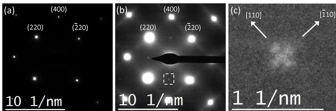
**Figure 5.25.:** SAED observation of S2 sample. (a) and (b) display the same pattern on two different intensity scale: the full range intensity for (a) and saturated intensity for (b). (c) zoom on the  $(0\bar{2}0)$  reflections.
