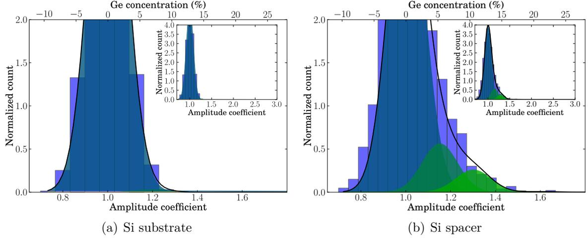
**Figure 4.20.:** Zoomed amplitude distribution (lower axis) and corresponding Ge concentration (upper axis) in the Si substrate and in the Si spacer in (a) and (b), respectively. The integrated count of the distribution have been normalized to one. The linear combinations of Gaussian functions are plotted with a black solid line on the histogram. The general view of the histogram are plotted in the insets. The histograms integrate about  $\sim 3000$  atomic columns for both distributions.
