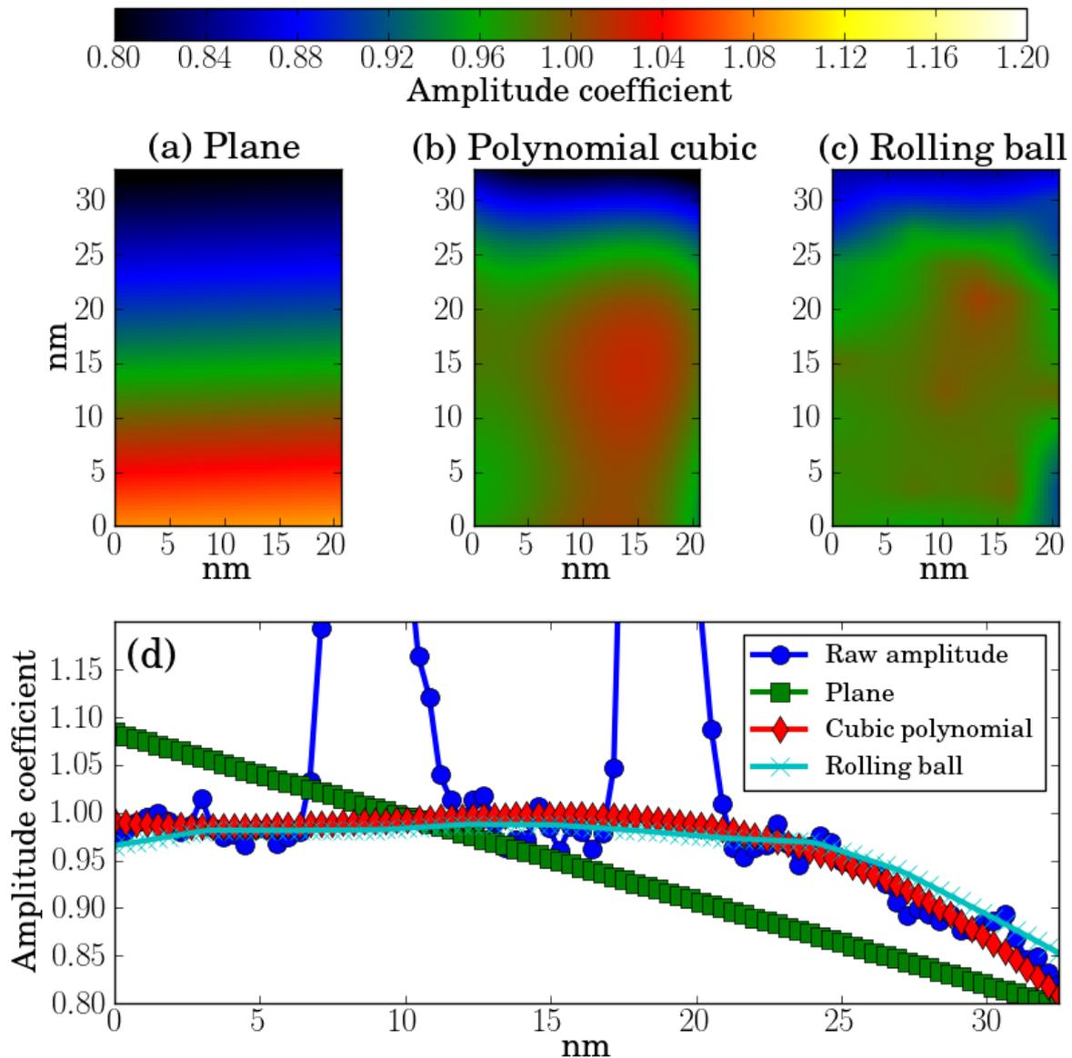
**Figure 4.18.:** Comparison of different background model for the amplitude map shown in Fig. 4.16(a). Analytic function (a) plane, (b) cubic polynomial and non-analytic (c) Rolling-ball background model. (d) Plot of the profiles of raw amplitude (blue dots), and model background: plane (green square), cubic polynomial (red diamond) and Rolling ball (cyan cross).
