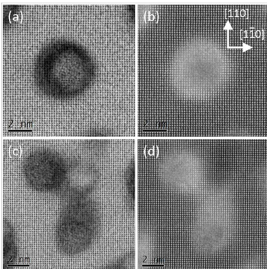
**Figure 5.9.:** (a) and (b) BF and ADF images respectively of the same emerging NCs with a straight shape. (c) and (d) BF and ADF images respectively of another NC exhibiting a Y shape with two emerging branches as revealed by APT observation shown in Fig. 5.7(c).
