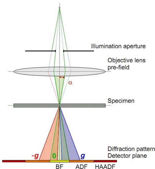
**Figure 2.12.:** Principle of STEM. The illumination aperture delimits the convergence angle, and the pre-field of the objective lens focuses the probe on the specimen. The scattered signal is collected by detectors as a function of the probe position, forming an image. Taken from [[Erni 10](#)].
