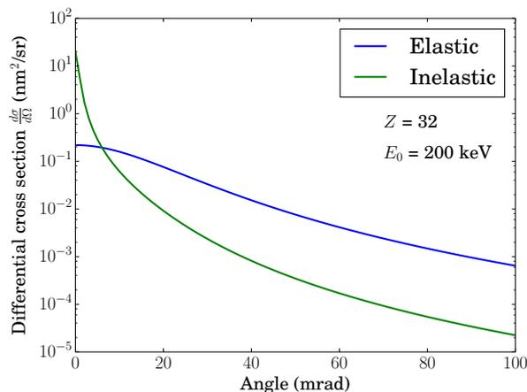
**Figure 2.2.:** Angular dependence of the differential cross sections for elastic and inelastic scattering calculated using Lenz model [Eger 11]. The calculation considers the scattering of 200 keV electrons by a Ge atoms.
