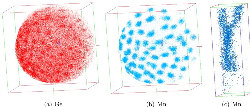
**Figure 5.7.:** Reconstructed volume of (a) Ge and (b) Mn obtained from APT experiment in top view. The volume in (a-b) are oriented along the growth direction. The position of the GeMn NCs can be recognized by the Mn-rich area in (b). (c) Side view of a junction of two GeMn NCs. Experiment performed by Pierre-Henry Jouneau, Bastien Bonafant from CEA INAC and Adeline Grenier from CEA LETI.
