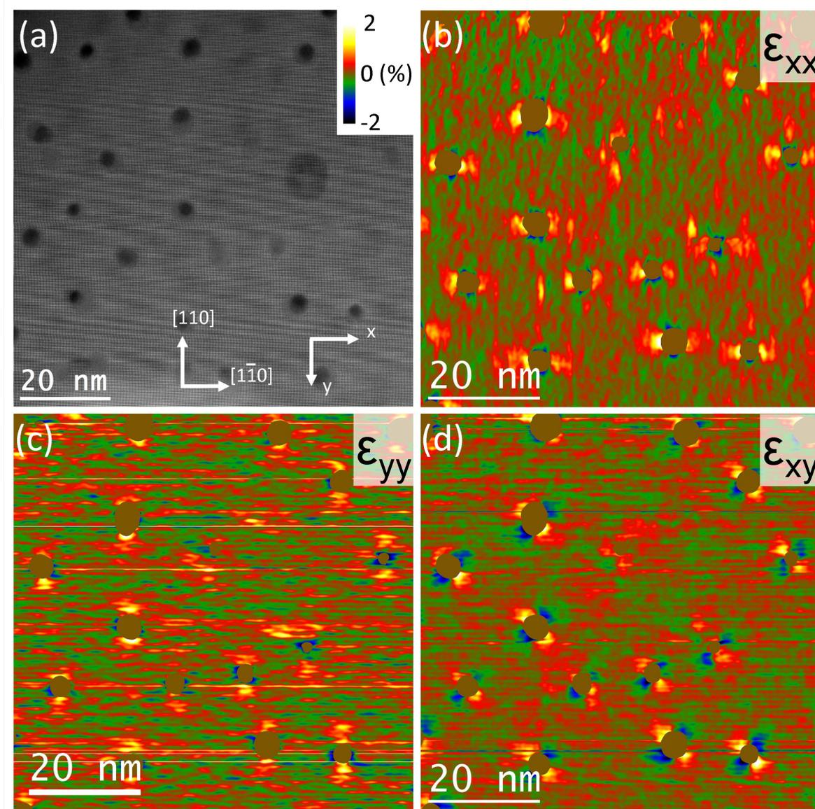
**Figure 5.30.:** GPA performed on HAADF-HRSTEM images of a  $\text{Ge}_{0.926}\text{Sn}_{0.014}\text{Mn}_{0.06}$  film in  $[001]$ -zone axis. (a) HAADF-HRSTEM images and corresponding (b,c) in-plane  $\epsilon_{xx}$ ,  $\epsilon_{yy}$  and  $\epsilon_{xy}$  strain maps.
