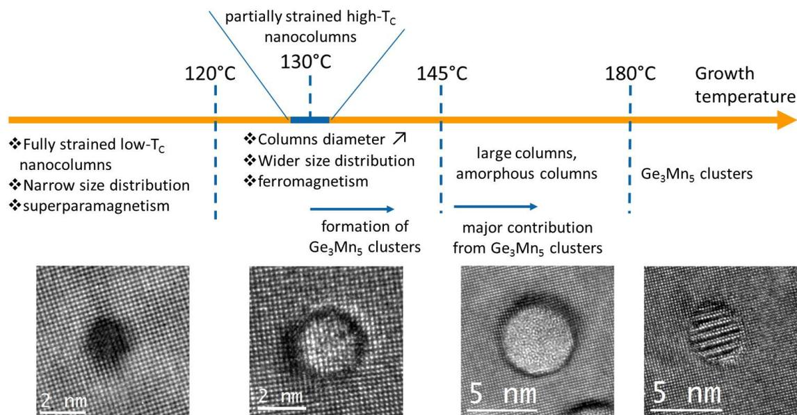
**Figure 5.1.:** Evolution of the GeMn NCs as a function of the growth temperature. Below a temperature growth of 120°C the NC are fully strained by the matrix. Between 120 and 145°C relaxed ferromagnetic NC are formed. Increasing the temperature leads to amorphous NCs and  $\text{Ge}_3\text{Mn}_5$  incoherent precipitates. Each kind of NC is illustrated by a corresponding HRTEM image in [001]-zone axis (plane view). Adapted from [Devi 08].
