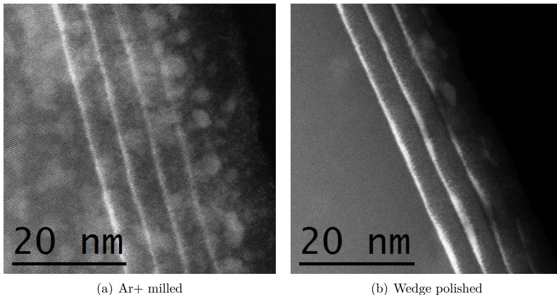
**Figure 2.27.:** HAADF-STEM image of Ge quantum dots in Si in [110]-zone axis (cross-section) showing the difference between Ar<sup>+</sup> ion-milling preparation (a) and wedge polished preparation (b). The specimen thickness is estimated to be  $\sim 10$  nm in both cases.
