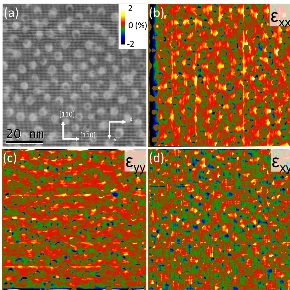
**Figure 5.19.:** GPA of the Ge matrix of a GeMn sample containing crystalline NCs. (a) Plane view 200kV ADF-HRSTEM images. (b, c, d)  $\epsilon_{xx}$ ,  $\epsilon_{yy}$  and  $\epsilon_{xy}$  strain maps. The position of the NC are reported in the strain map by using a threshold on the amplitude map of the Fourier component (not shown here).
