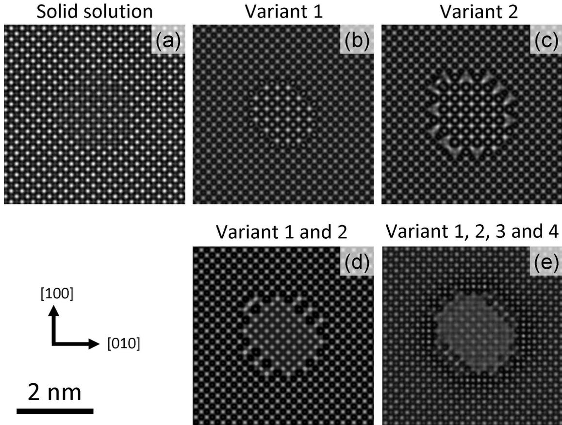
**Figure 5.15.:** HRTEM image simulation of GeMn NC with different structure model. (a) Solid solution. (b)  $\alpha$ -phase with the variant n°1. (c)  $\alpha$ -phase with the variant n°2. (d)  $\alpha$ -phase with the variants n°1 and n°2. (e)  $\alpha$ -phase with the variant n°1, 2, 3 and 4.
