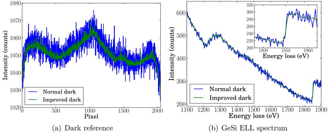
**Figure 2.23.:** (a) Normal and improved dark-current reference and (b) the impact on typical raw EELS spectrum of a SiGe specimen with Ge  $L_{2,3}$  and Si K edges. The improved dark current reference  $\bar{D}_i$  was averaged over  $i = 400$  dark current reference  $D_i$  acquisitions.
