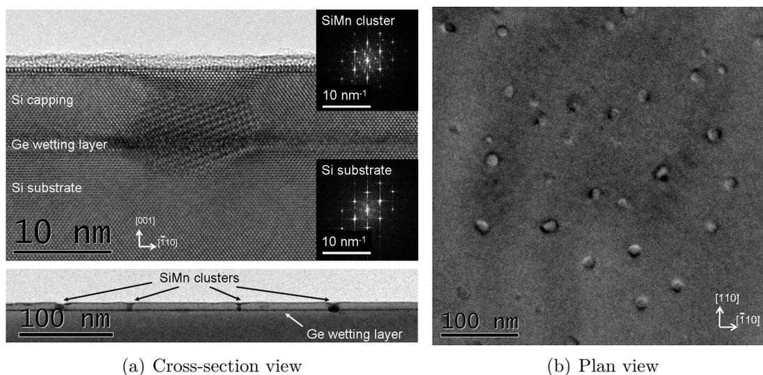
**Figure 4.29.:** HRTEM observations of a unique GeMn WL. (a) Cross-section view images in [110]-zone axis showing SiMn precipitates, which can be recognized with the Moiré pattern on the top HRTEM image. The dark area on the bottom bright-field TEM image correspond to the Moiré pattern. The FFT of SiMn precipitates and the Si substrate are displayed in the insets. (b) Plan-view bright-field TEM image acquired in the [001]-zone axis shows the in-plane distribution of SiMn precipitates.
