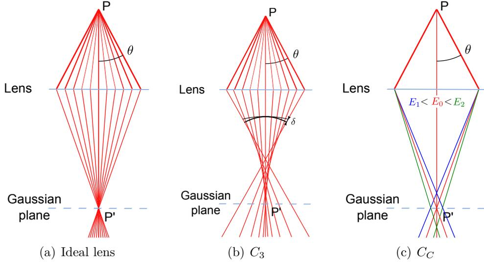
**Figure 2.4.:** (a) Ideal lens focused all rays coming from point  $P$  of the object plane to another point  $P'$  of the image plane. Real lens with spherical aberration (b) and chromatic aberration (c), the point  $P$  is imaged as a disk in the Gaussian plane.
