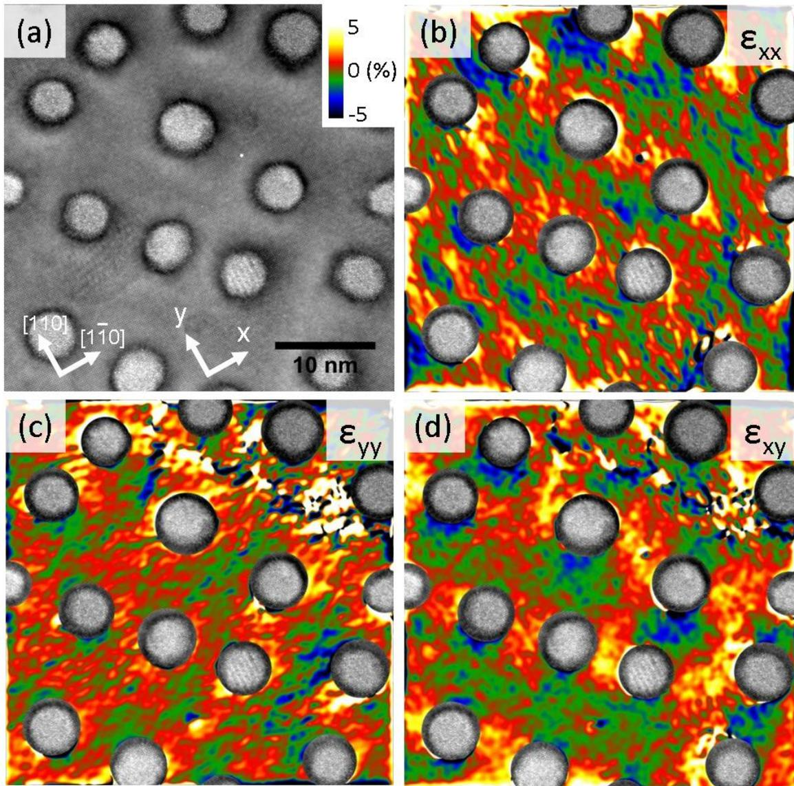
**Figure 5.18.:** GPA of the Ge matrix of a GeMn sample containing amorphous NCs. (a) Plane view 400 kV HRTEM images. (b, c, d)  $\epsilon_{xx}$ ,  $\epsilon_{yy}$  and  $\epsilon_{xy}$  strain map. Piece of image have crop in the HRTEM and paste on the strain map as guide to the eye.
