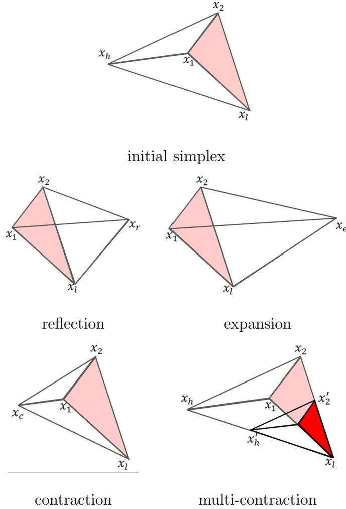
Figure 5.4: Simplex transformations in the Nelder-Mead algorithm.
