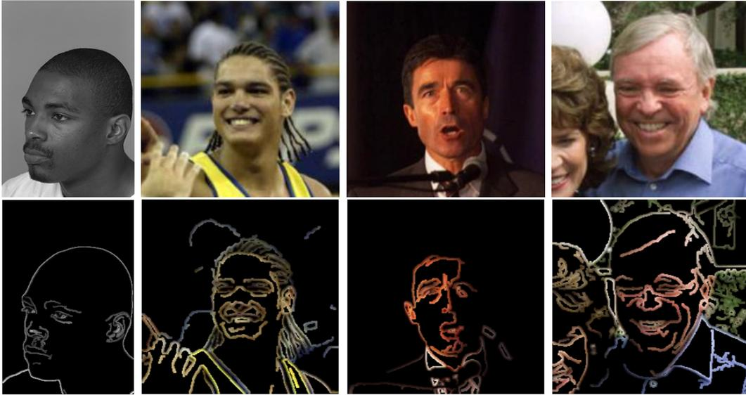
Figure 5.3: Edge responses (second row) superimposed on the original images.
