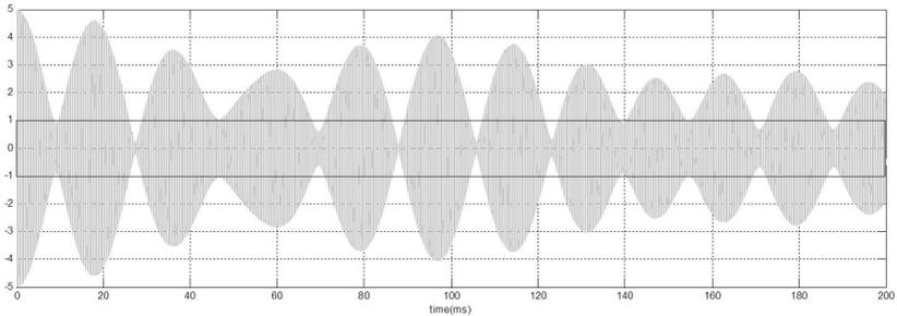
(b) The envelop of the CC-T output in the case of frequency error
