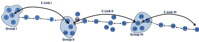
(b) MH-CC path after fixing the failure:  $N_{14}$  is substituted by  $N_{12}$
