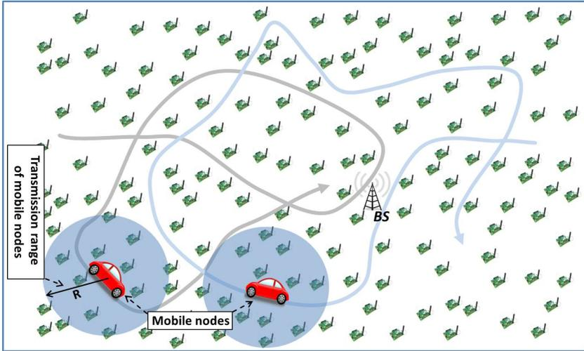
**Figure 2.12:** Data communication in mobile WSNs
