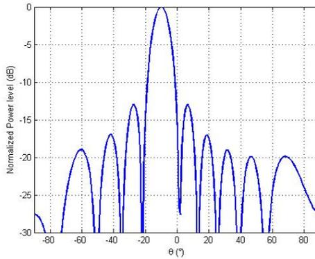
(b) Corresponding beam-pattern to a Uniform Linier Array of 10 antennas
