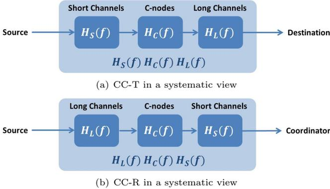
**Figure 3.4:** Comparison of CC-T and CC-R in a systematic view
