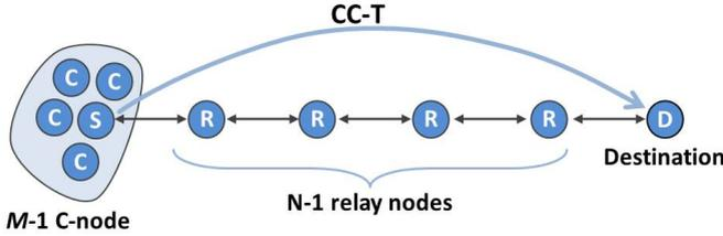
**Figure 3.6:** WSN model considered to extract the minimum number of C-nodes
