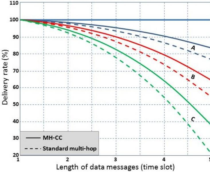
**Figure 4.10:** The impact of MH-CC on the reliability for different lengths of messages and mobility modes
