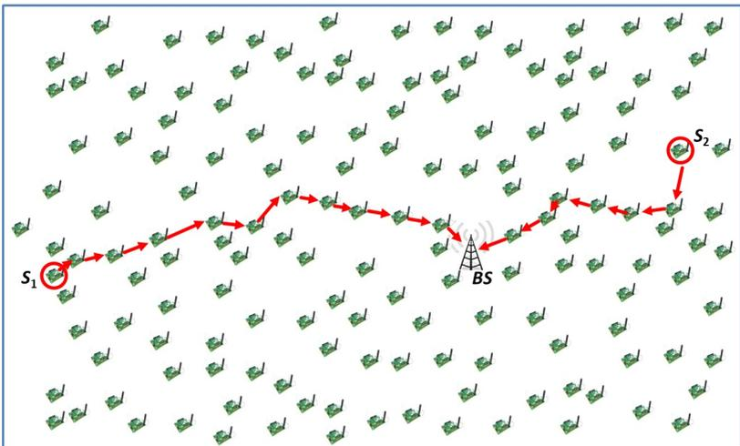
**Figure 2.4:** Data communication in multi-hop WSNs
