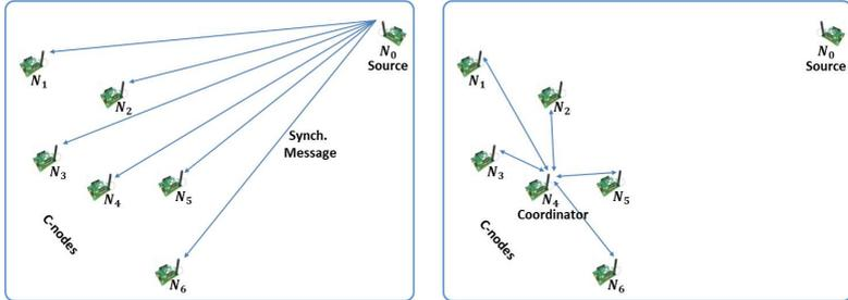
(a) C-nodes receive the signal of the source (b) C-nodes interact to the destination for synchronization
