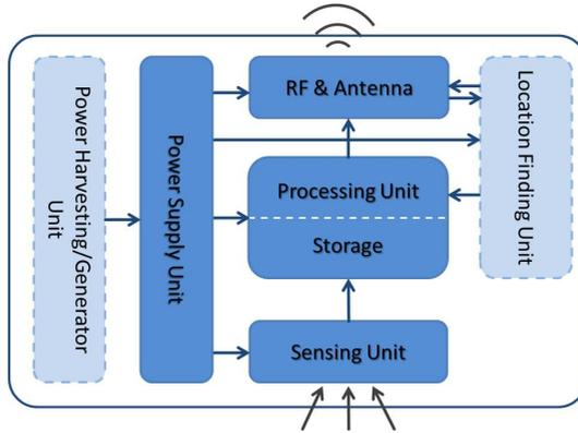
Figure 2.1: A view of a typical sensor node
