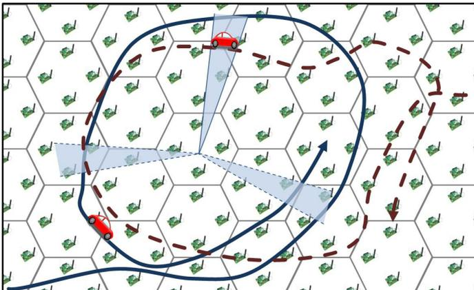
**Figure 5.3:** Sensor nodes at each cluster use CC-R to detect a mobile node and then use CC-T for data communication
