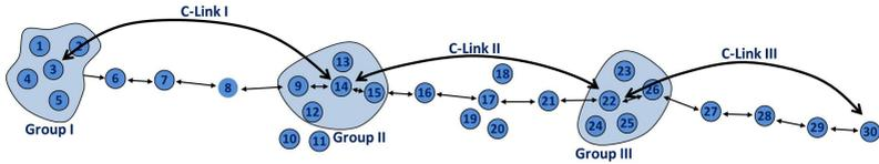
(a) MH-CC path before the failure of  $N_{14}$  as CR-node
