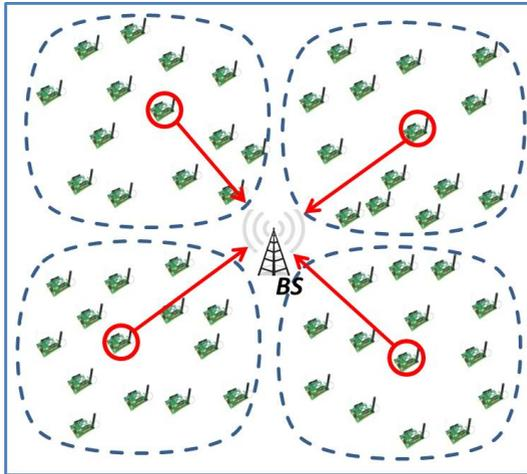
**Figure 2.3:** Hierarchical data communication in cluster-based WSNs
