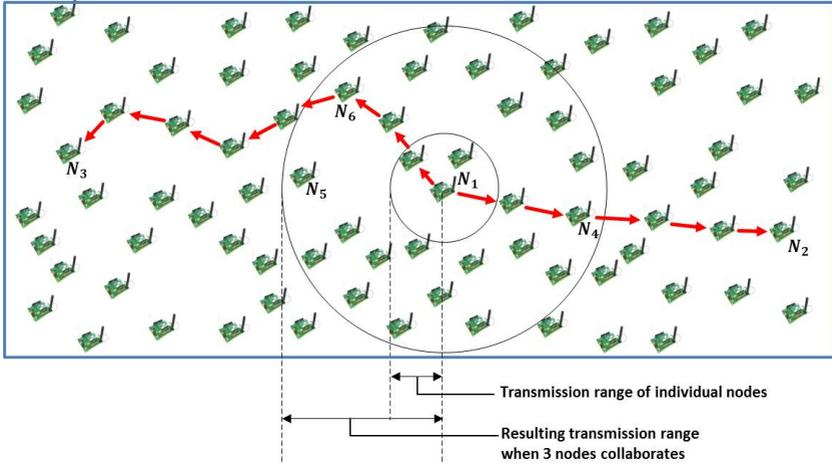
**Figure 4.2:** Comparison of the number of potential relay nodes in MH and MH-CC (for  $M = 3$  C-nodes)
