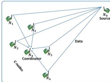
(c) C-nodes relay the signal of the source to the destination after phase modification
