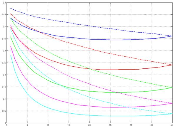
**Figure 3.12:** Comparison of the minimum number of C-nodes to gain different levels of BER for the proposed and conventional methods
