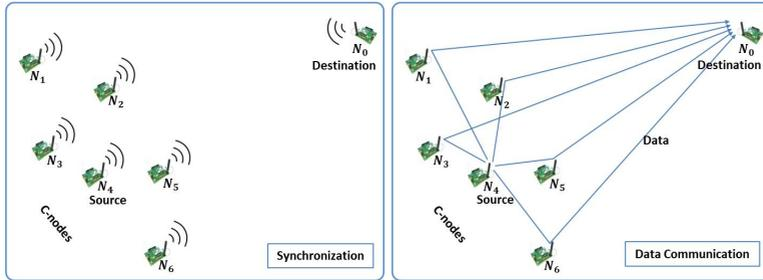
(a) Synchronization step: appropriate phase shifts for C-nodes are achieved and (b) C-nodes modify their carrier phases and relay the signal of the source simultaneously through the destination
