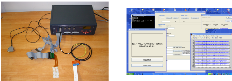
Figure 3.5 – EMG Recorder and Recording Software screenshot for the electrode array setup
