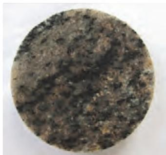
**Figure 1:** Sample AD-1 for electromigration measurement.
