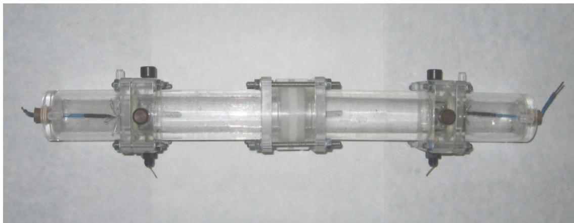
**Figure 6:** The photo of inlet compartment, outlet compartment and sample mounted between as a part of the through-electromigration apparatus (UJV Rez, a. s. concept; reproduced from Löfgren et al., 2009).
