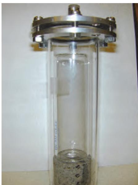
**Figure 3:** The specially made holder for gas adsorption measurements of drill-core sections.
