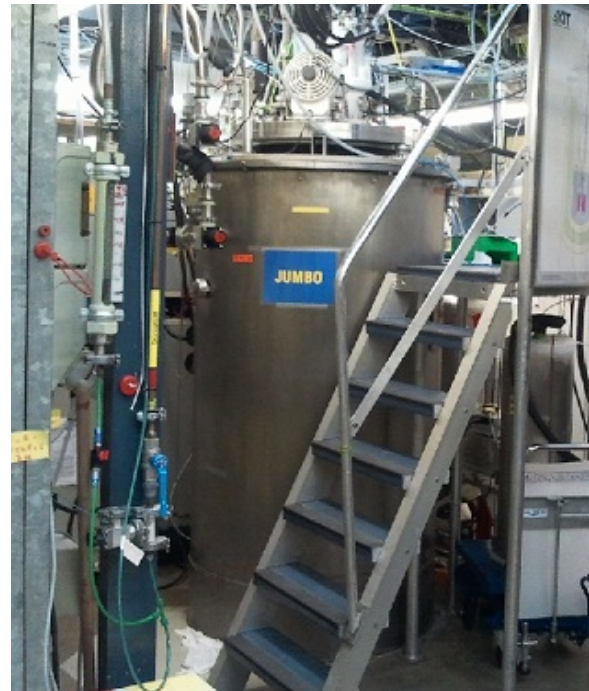
Figure 6.5.: JUMBO superconducting magnet [RHS00]. The coil is located in a cryostat filled with liquid helium. An additional warm tube can be inserted into the cryostat which insulates the sensors from the helium. This allows measurements at temperatures up to room temperature.
