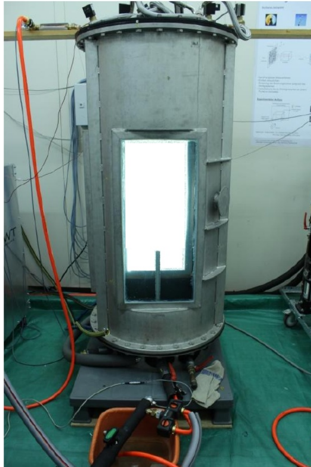
Figure 7.9: Picture of the tank with inlet pipe
