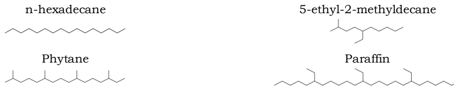
Figure B-1: Molecular structure of the chosen branched alkanes in comparison with linear n-hexadecane.
