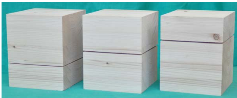
Figure 5: Glulam test blocks for compressive force measuring in the height of 50 mm, 100 mm and 150 mm.
