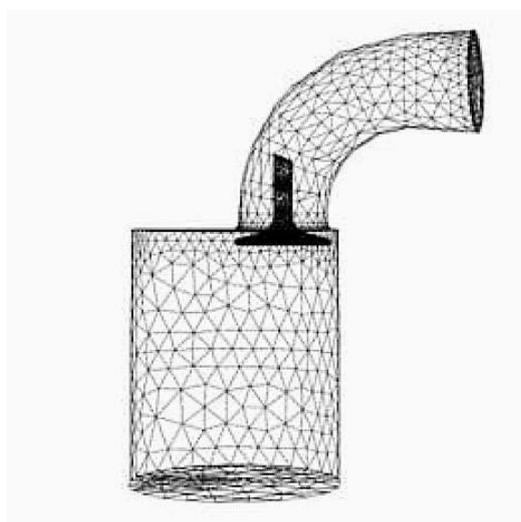
Figure 2.6 Grid structure in ANSYS CFX [2]
