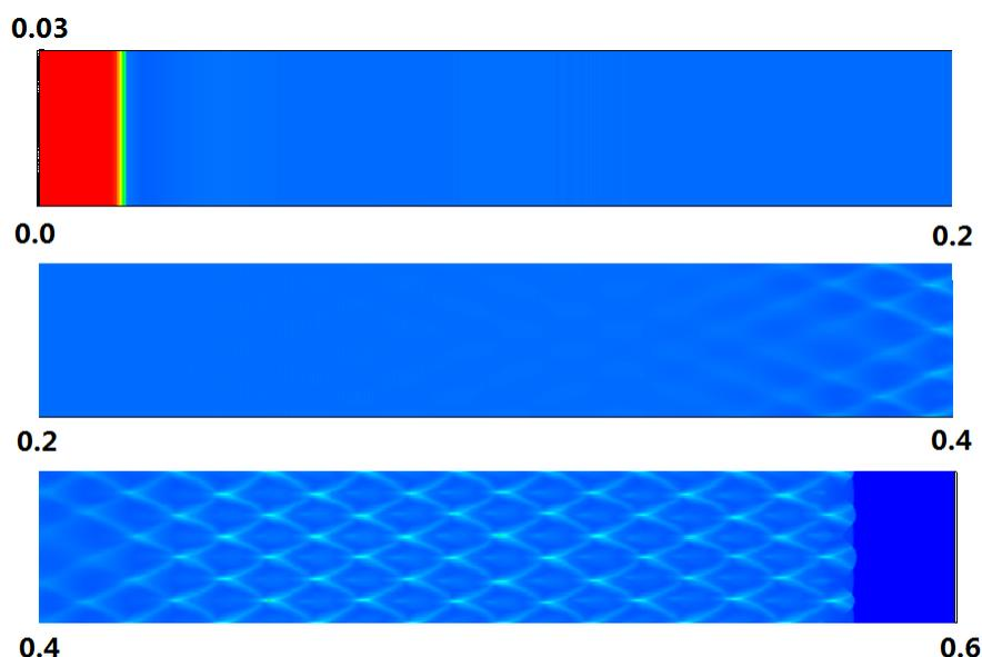
Figure 5.33 Numerical smoke-foil record for 2D detonation with ALMR
