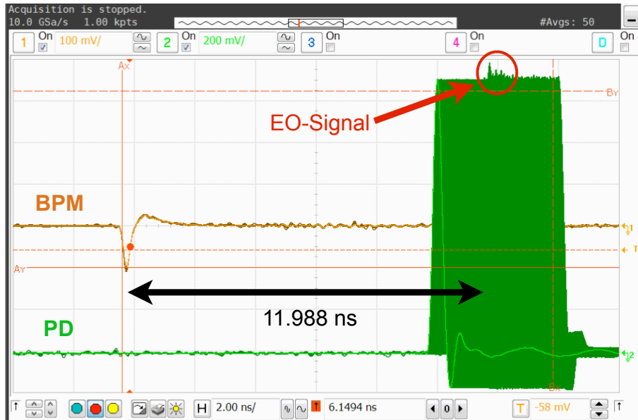
Figure 5.14: Screenshot of the first temporal overlap seen with an infinite persistence scan. The oscilloscope was triggered on the BPM signal. The laser delay was scanned while keeping infinite persistence switched on for the photodiode signal. This superimposes multiple wave forms in the same view, drawing the most recent one in a brighter color. This allows us to spot an EO signal directly on the screen without having to read out every single wave form for every delay and analyzing it.
