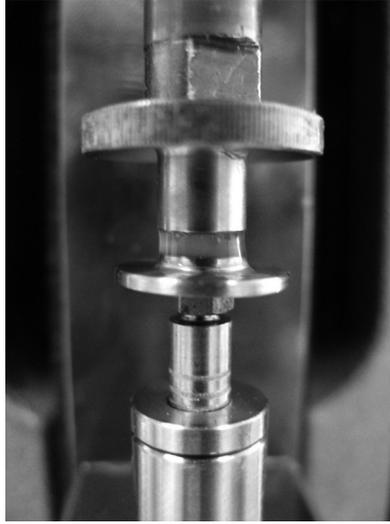
**Figure 5.6.** – The newly designed axial force measurement device for the CaBER with a sample loaded. The plates have a diameter of 6 mm. The lower plate geometry is directly screwed into the force transducer and fixed with a counter nut.
