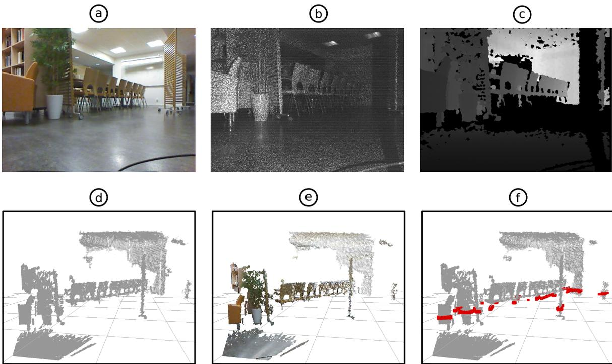
Figure 3.6: Available data streams using the Kinect camera
