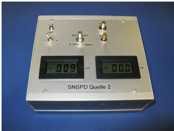
Figure 3.11: Image of the low noise current source
