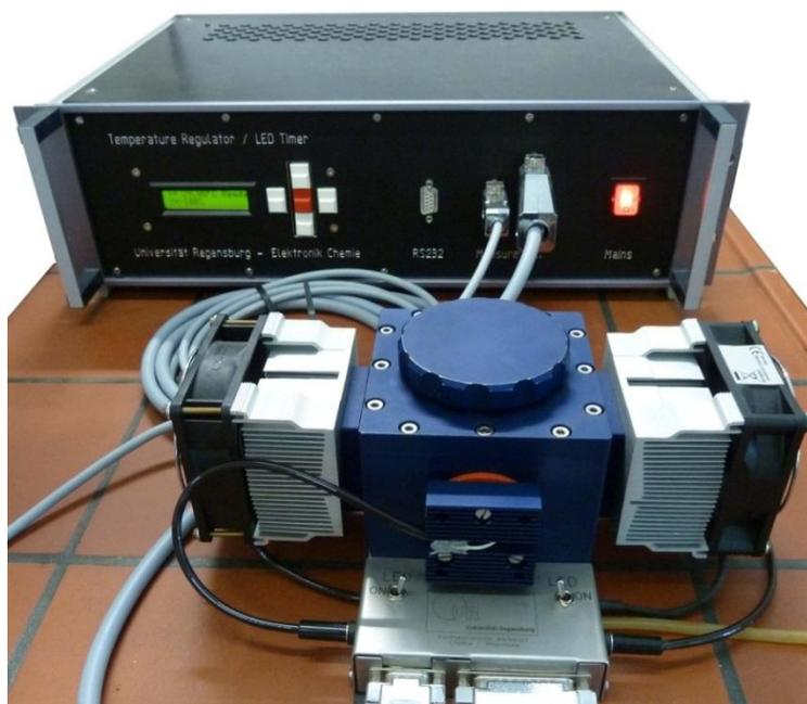
**Figure 25:** LED-illuminator with peltier temperature control unit, stirrer and control device.
