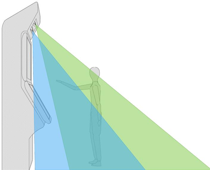
Figure 5.18: The technical setup of the distance dependent display along with the overlapping fields of view of the two Kinect cameras.
