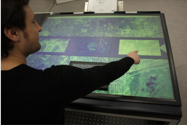
Figure 5.7: A hand gesture consisting of a single, stretched out finger allows to trigger clicks and choose between different map layers, for example.
