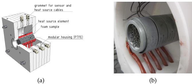
Figure 3.11: Three dimensional design model of the test section of the test rig, with foam samples, heat sources and modular housing elements; the temperature sensors are omitted here.
