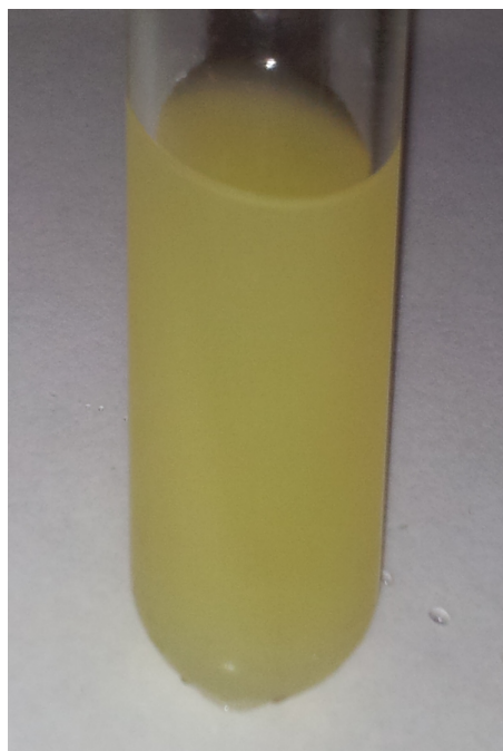
Figure A.5: Picture of the suspension of maleimide-functionalized microspheres in a solution of RAFT-polymer (here PDMAA) in DCM prior to irradiation.
