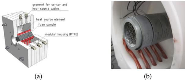
**Figure 3.11:** Three dimensional design model of the test section of the test rig, with foam samples, heat sources and modular housing elements; the temperature sensors are omitted here.
