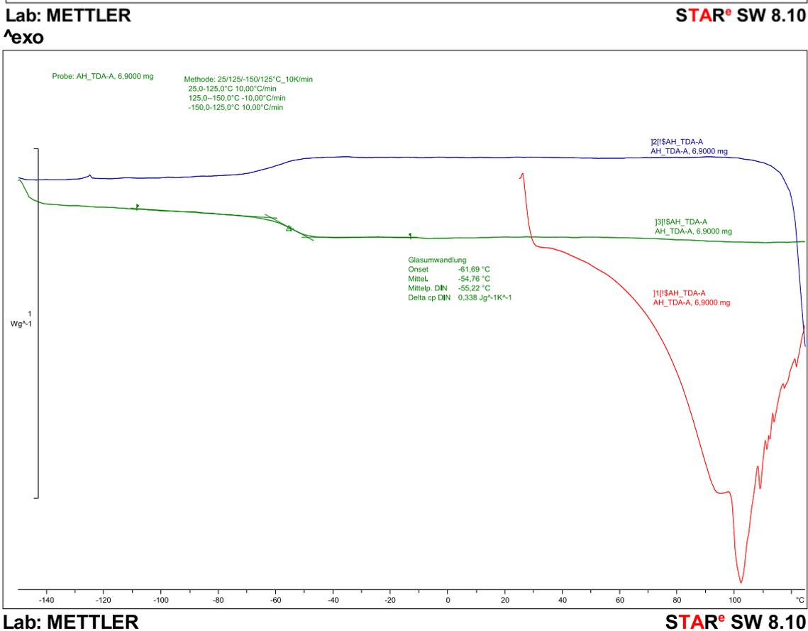
**Figure S29** Differential scanning calorimetry of pPHA (upper part) and pTDA-A (lower part). The glass transition temperatures are summarized in Table 2.1.
