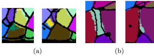
Figure 6.1.: Close ups of two grains in two cross sections of the DCT reconstruction. Both the brown grain in the lower part of (a) and the green grain in the center of (b) exhibit boundaries which are close to parallel to the section resulting in a large shift and irregular shape when going from one section to the other.
