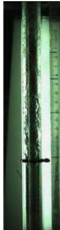
Fig. 6: COSMOS-L test facility for the investigation of the influence of surface structure on CHF
