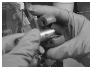
cut the top and the bottom of the case with a pipe-cutter
