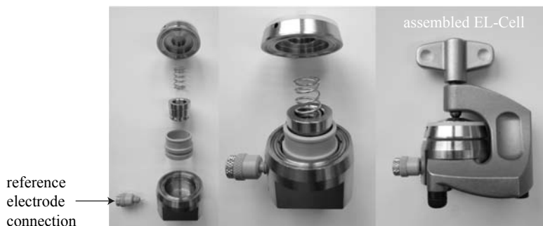
Figure 4.1: EL-Cell housing with integrated reference electrode connection [135].
