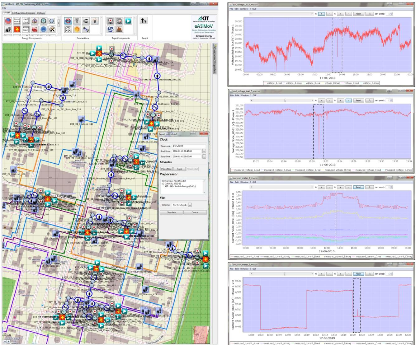
The model contains the available grid component specifications. The active power values based on the 10 minutes smart meter power consumption data at KIT-CN and the 5kHz sampled high rate EDR voltage data are used as input for the simulation model. GridLAB-D manages the data synchronization for the multi-rate input time series and performs the calculation of the power flow with
