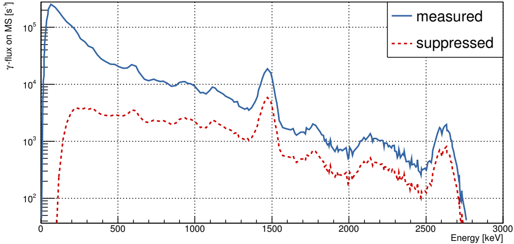
Figure 3.8.: Environmental radiation-spectrum KATRIN hall Measured spectrum of environmental gamma radiation in the KATRIN hall (solid line) and spectrum of dampened radiation inside the main spectrometer (dashed line). Some \gamma -peaks of ^{40}\text{K} (1.46 MeV), ^{208}\text{Tl} (2.61 MeV) and ^{214}\text{Bi} (0.58 MeV) are clearly visible in both spectra. Energies taken from [126].
