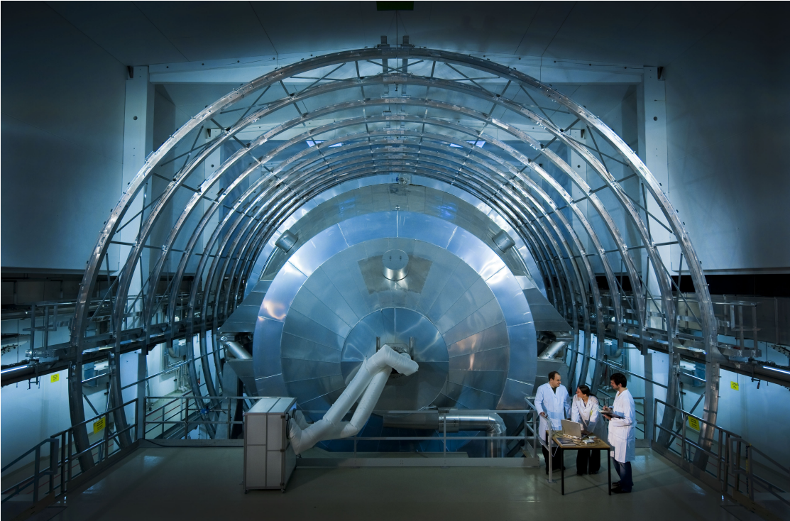
Figure 2.10.: Photograph of the main spectrometer including the air-coil mounting-structure. The author can be seen on the very right.
