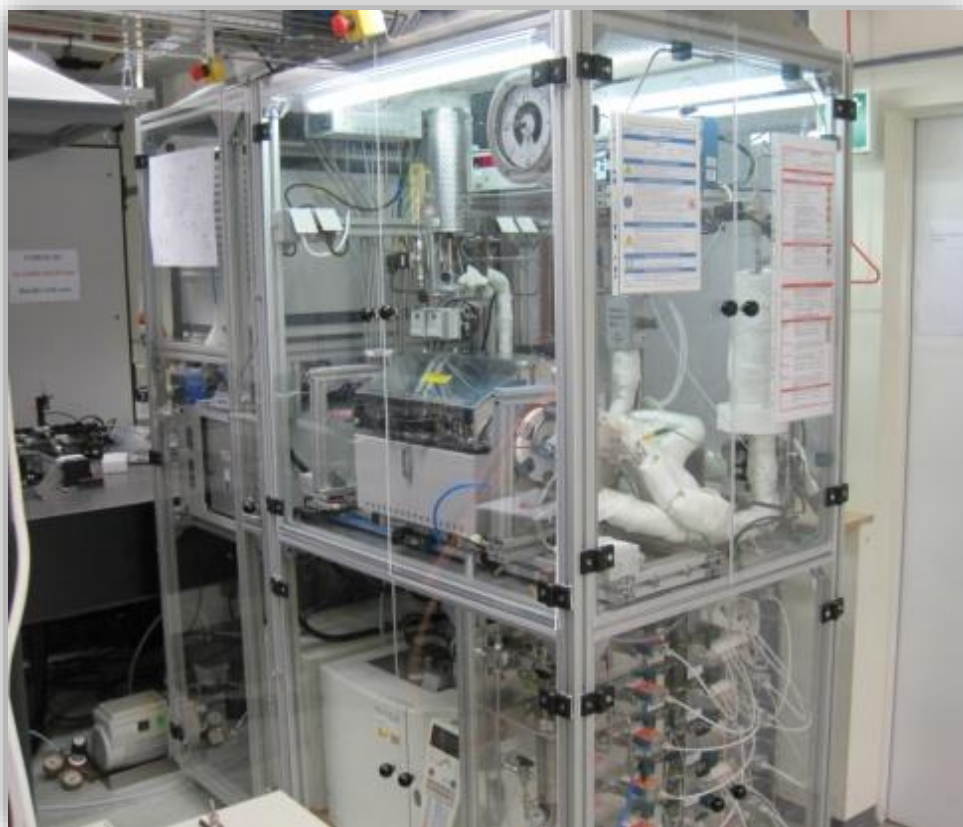
Figure 3.3 Picture of the fully assembled reactor setup CPOX 2.
