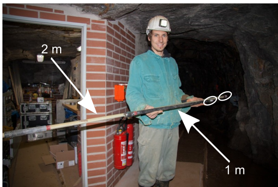
(c) 1 and 2 m long geophone anchors
