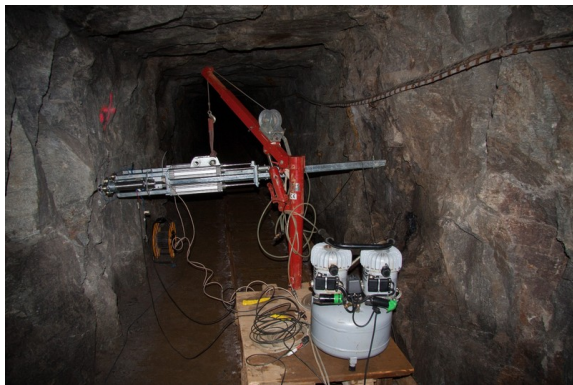
(a) Magnetostrictive double vibrator
