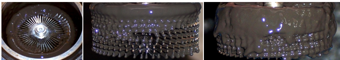
Figure 5-12 left: particle cake at a low particle amount from the top; middle: particle cake at low particle amount from the side; right: completely plugged filter at high particle amount
