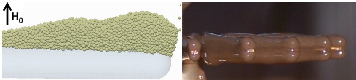
Figure 4-10 left: simulation of the particle deposition of weakly magnetic particles on a magnetic wire; right: deposition of weakly magnetic particles in the MEC and removing from the magnetic field results in a similar deposit compared to the simulation
