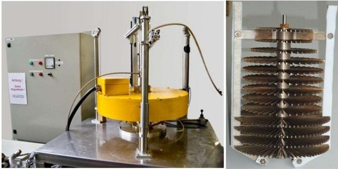
Figure 5-20 left: the MEC set up inside the magnet; right: the matrix and peeler knives [Lindner'13]
