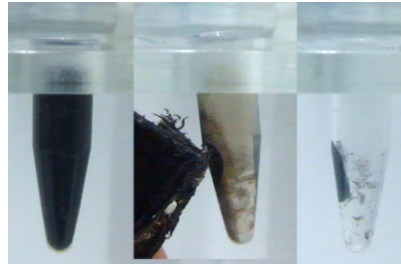
Figure 6-4: Treatment of magnetic particles in a \mu\text{l} reactor
