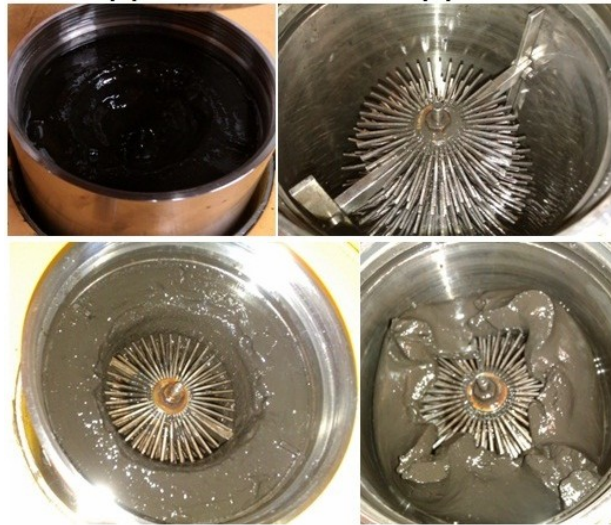
Figure 5-25 top left: the centrifuge is filled with particles after the test; top right: the effectively cleaned centrifuge shows only few particles left close to the axis ; bottom left: inefficient discharge without use of the peeler knives shows a flushed center but dense cake; bottom right: inefficient discharge using a low volume flow shows a clear center and a cake solved from the wall but not discharged [Lindner'13]
