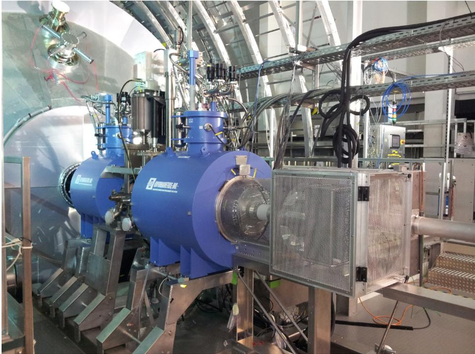
**Figure 3.1: Detector system completely assembled**, prior to its connection to the main spectrometer. The detector system constitutes the downstream end of the KATRIN experiment. In the background, the main spectrometer is visible. Picture adapted from [Har12].
