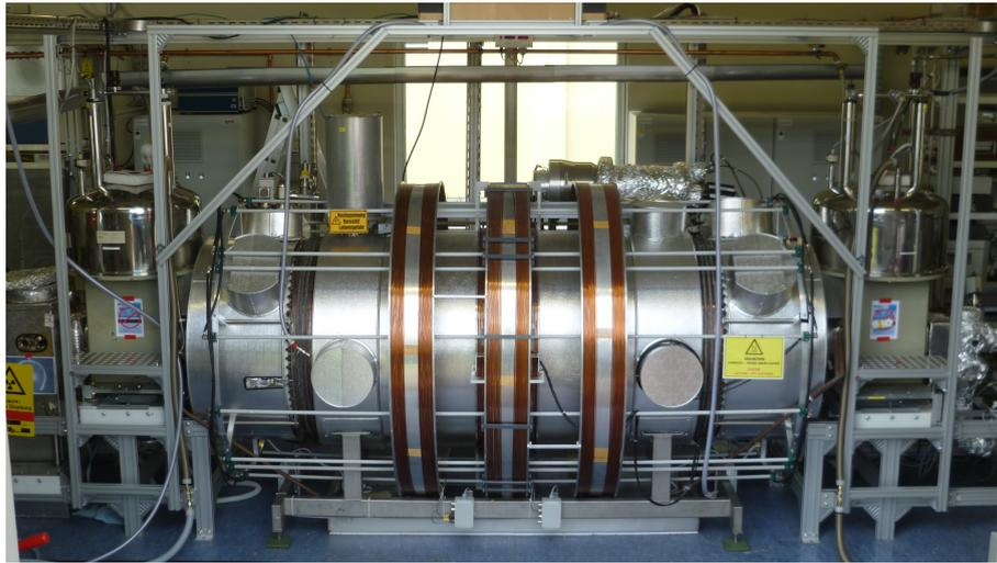
**Figure 2.5: Monitor spectrometer.** The monitor spectrometer is positioned separately from the KATRIN beam line. There, the magnetic guiding field is provided by two superconducting solenoids coaxially arranged on both ends of the spectrometer and by four air coils surrounding the vessel. The middle air coil consists of two layers.
