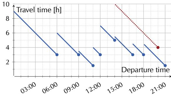
**Figure 4.6.** Piecewise linear travel time function.
