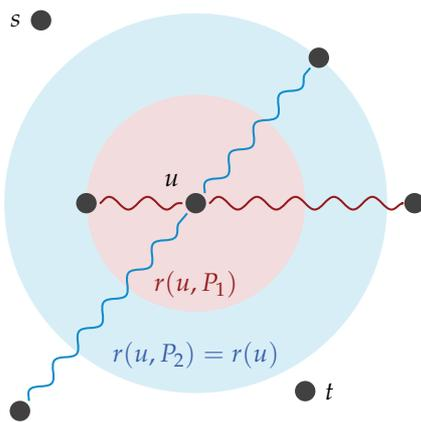
**Figure 2.6.** Reach of vertex  $u$  determined by the paths  $P_1$  (red) and  $P_2$  (blue). An  $s$ - $t$  query may prune  $u$ .
