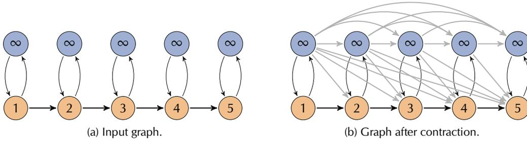
**Figure 5.6.** Contracting only route vertices in the realistic time-dependent model [PSWZ08]. The top row are stop vertices, and the bottom row are route vertices contracted in the order depicted by their labels. Grey arcs represent added shortcuts. Note that these shortcuts are required as they incorporate different transfer times (for entering and exiting vehicles at different stops).
