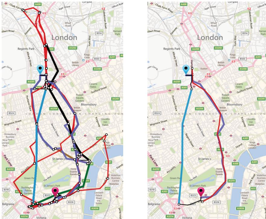
**Figure 5.13.** Exemplary multicriteria multimodal query on London with criteria arrival time, number of transfers, walking duration, and cost. The left figure shows the full Pareto set (65 journeys), while the right figure shows the three journeys with highest score. Each dot represents a transfer and included transportation modes are walking (thin black), taxi (thick purple), buses (thin red), and tube (other thick colors).
