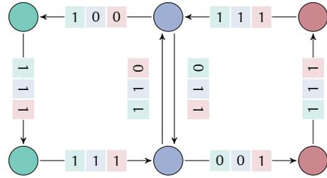
Figure 2.5. Arc flags for a small graph.
