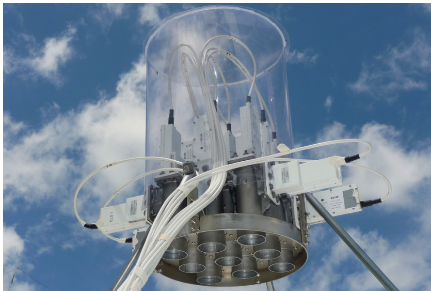
FIG. 4.7 • Close up of one of the nine feed cameras mounted in the 3.4 m reflectors. The final configuration is shown, in which the four corner feed horns are equipped with two LNBs for dual-polarised measurements.
