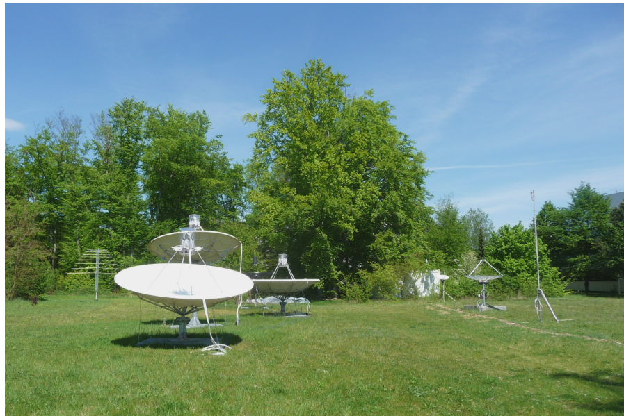
FIG. 4.4 • Photograph of the CROME experiment in one of its last configurations (May 2012). The three largest antennas, 3.4 m reflectors, are operated in the extended C band (3.4 GHz to 4.2 GHz) and are the leading instruments of the experiment. On the left, a VHF LPDA antenna (30 MHz to 80 MHz) that was reused from the LOPES' experiment is visible, three others were distributed around the area. Two smaller reflectors, one in the background (black), one on the right hand side (metallic), were used for measurements in the L band (1 GHz to 2 GHz). A VLF antenna ( \sim 100 kHz to several MHz) was mounted on the long pole seen on the far right.
