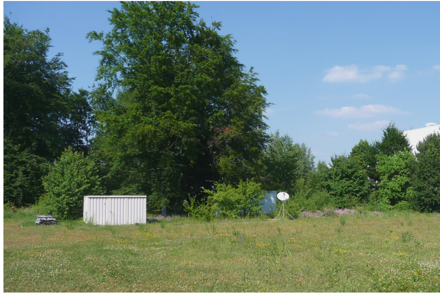
FIG. 4.3 • Photograph of the CROME experiment in its initial phase (June 2010). The first antenna, a 90 cm reflector operated in the lower K_u band (10.7 GHz to 11.7 GHz), is visible in front of the DAQ container. The container on the left, part of the Piccolo trigger cluster, was removed later.
