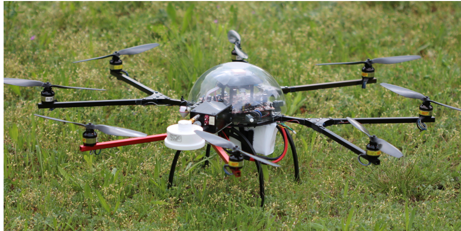
FIG. B.2 • Octocopter with the C band emitter (black case with white, downward-pointing spiral antenna) attached to the front arm (coloured red for identification during flight). The eight rotors are arranged coplanarly on a circle with a diameter of about 80 cm. The sensors and electronics are protected by a cover made of polyester. A lithium-ion polymer battery with an energy content of 150 W h (white) is attached to the baseplate between the landing gear.
