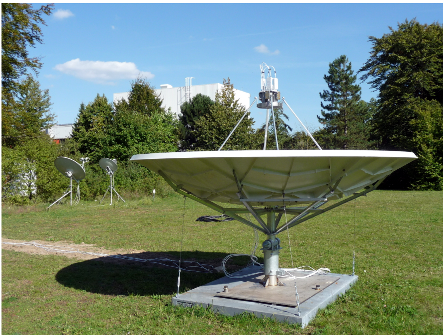
FIG. 4.6 • Prime focus 3.4 m reflector with custom-made four feed C band camera. The two reflectors shown in Fig. 4.5 are visible in the background.
