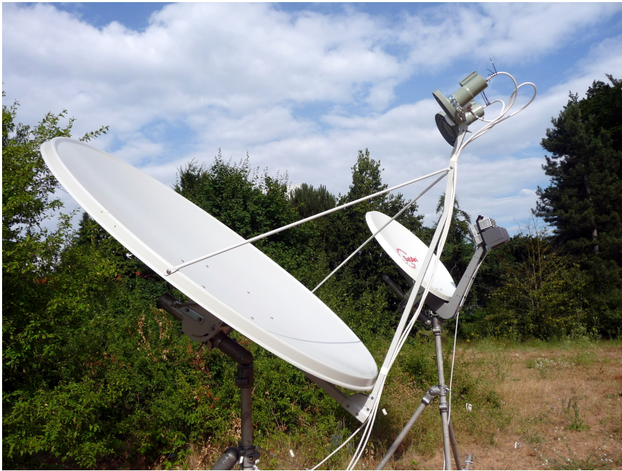
FIG. 4.5 • Offset-fed 150 cm reflector with one central K_u band feed and two outer C band feeds (foreground), and 90 cm reflector with two K_u band feeds (background).
