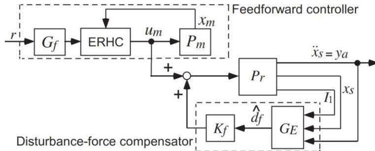
**Figure 2. Block diagram of the 2DOF electro-dynamics shaker controller [8]**
