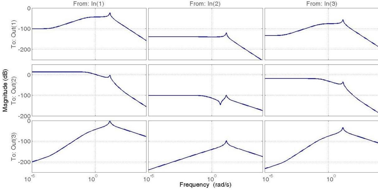
Figure 3. Bode diagram of the drivetrain open loop response
