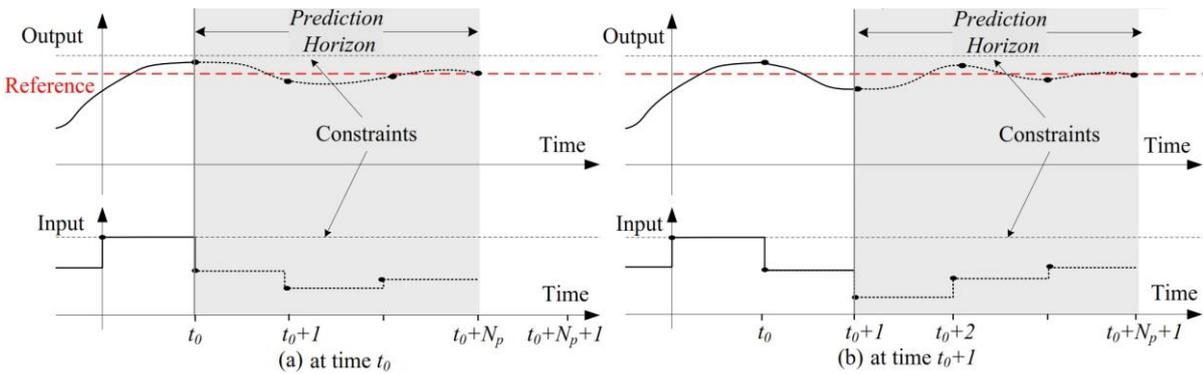
Figure 4. Illustration of the receding horizon of RHC methods [10]
