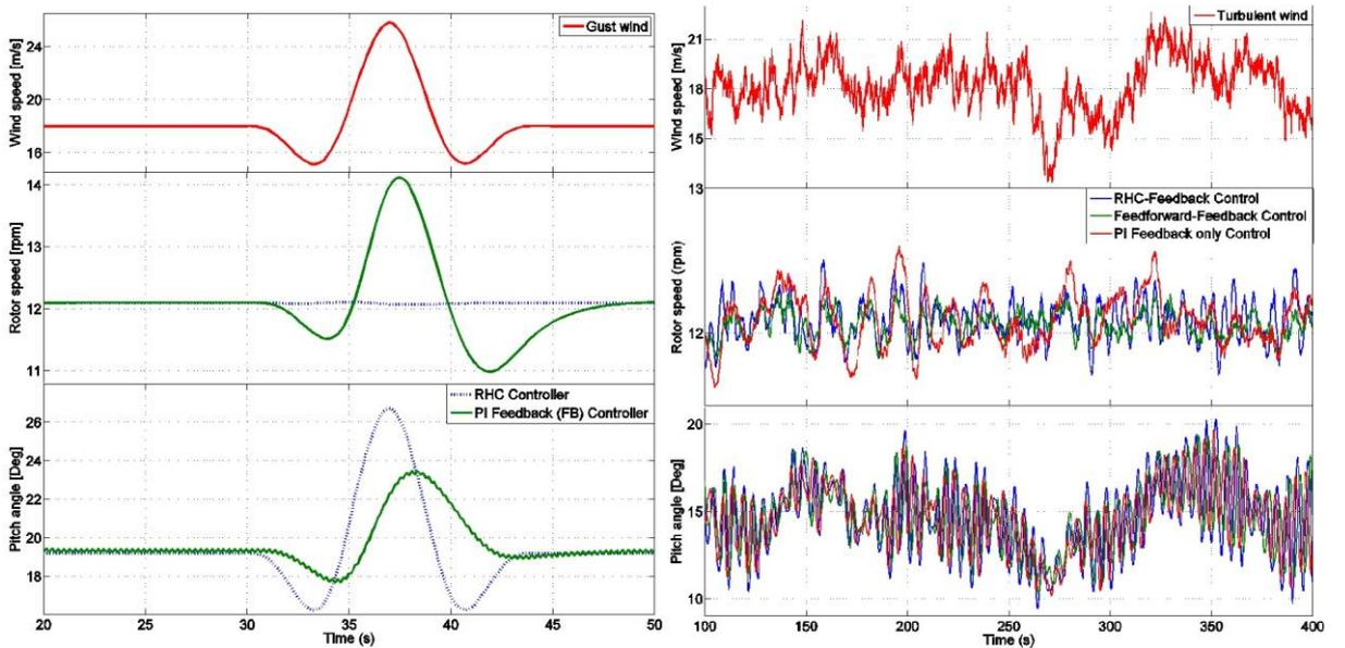
Figure 5. Simulation result with (left) gust wind (right) turbulent wind
