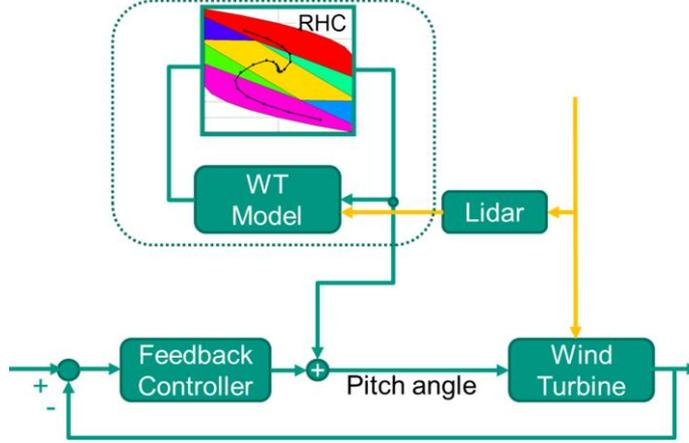
**Figure 1. System diagram of the 2DOF RHC/FB controller for the active pitch control of wind turbines, green represent the control signal, yellow represents the wind signal**
