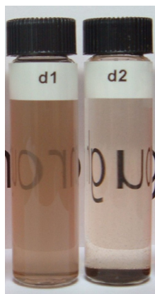
Figure 6.10: Suspensions synthesized from aqueous iron acetate solutions before (left) and after allowing sufficient time for sedimentation (right). No further changes were observable over a period of several months. Synthesis conditions: \phi_m = 0.1 , \dot{m}_{total} = 6.07 kg/h, c_{product\ Fe} = 0.001 mol/L.
