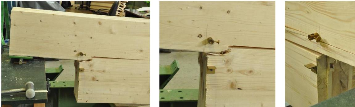
Figure 9: Shear failure in the crossing areas next to the corner of the notch
