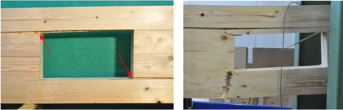
Figure 7: Shear failure in the crossing areas in specimen H50-4 (left), bending failure in the residual cross section below the hole in specimen H40-1 (right)
