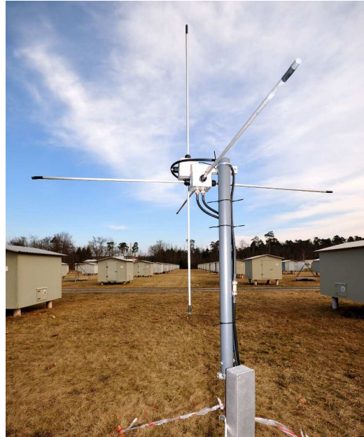
Figure 3.7.: Photography of a tripole antenna as used for LOPES 3D.
