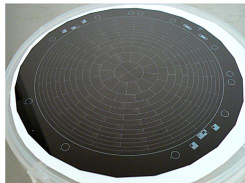
**Figure 2.7:** 148 pixel silicon wafer, each pixel having equal surface area.
