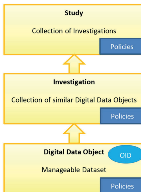
Figure 1 The hierarchical base metadata structure of the KIT Data Manager is based on the Core Scientific Metadata Model (CSMD).
