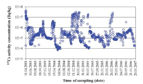
Figure 1: History of <sup>137</sup>Cs activity concentration in the pit with the cleaning tank of Unit 2.
