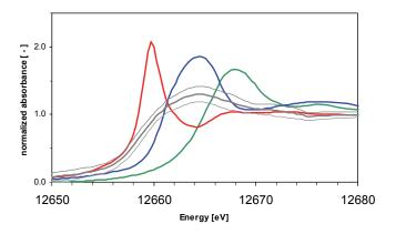
*Figure 4*: Average smoothed Se K-edge XANES spectra from all measurements recorded on the spent fuel samples from the same fuel pellet (thick grey line) and envelope of all individual spectra (thin grey lines) compared with the Se K-edge XANES spectra recorded on several Se reference compounds (red = Se(0), blue= Se(IV)O<sub>2</sub>, green =  $Na_2Se(VI)O_4$ ).
