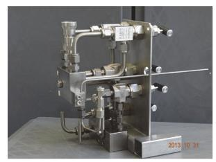
Figure 2: Manufactured autoclave head.
