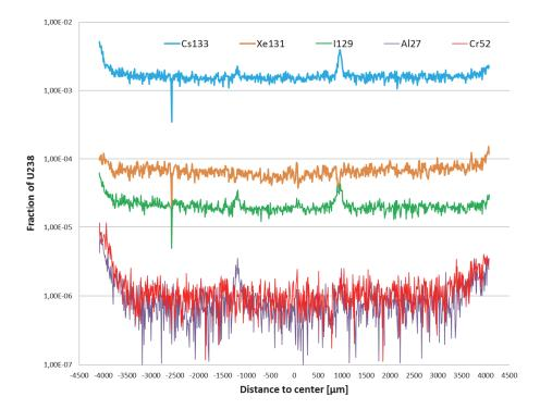
Figure 6: Ablation profiles on 5A2 along the red dashed track in figure 5 (60 µm beam).
