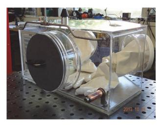
*Figure 3:* Glovebox for oxygen-free welding ( $\approx$ 7ppm  $O_2$  and <1ppm  $H_2$ ) of Ti parts.
