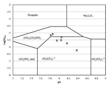
*Figure 5:* Speciation diagram of uranium in the studied experimental conditions (NEA and CHESS databases were used for the calculation). Measured uranium concentrations for each sample are also included.
