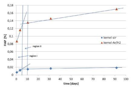
Figure 3: FIAP <sup>90</sup>Sr (%) vs. time under oxic and under anoxic/reducing conditions.
