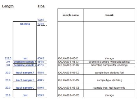
*Figure 1:* Segment cutting plan of the selected UO<sub>2</sub>BWR fuel.
