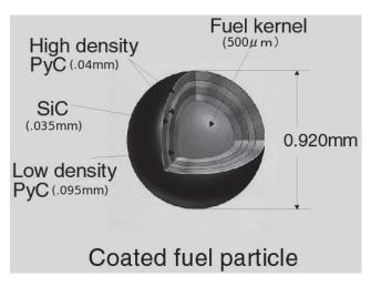
Figure 1: Design of a TRISO coated fuel particle.
