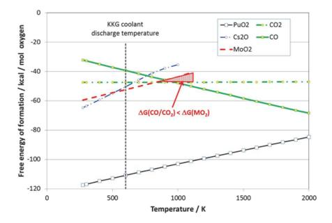
**Figure 2:** Free energy of formation for carbon oxides,  $Cs_2O$ ,  $MoO_2$  and  $PuO_2$ . The vertical dashed line indicates approximately the surface temperature of the cladding, the red triangle shows the temperature region where  $\Delta G_f$  of the carbon oxides are below those of  $MoO_2$ .
