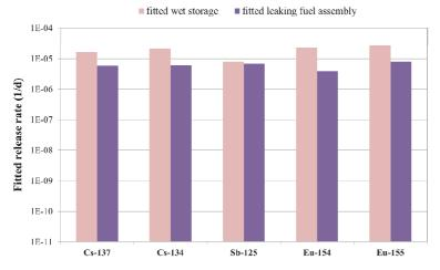
Figure 4: Comparison of the fitted release rate of long lived isotopes.
