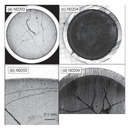
*Figure 3: Exemplary section images of initially 3.8 wt.%* <sup>235</sup>U enriched pellets of fuel segments N0203 and N0204. Ceramography images of N0203 are taken from F. Weiser (KfK-HZ). Detail images (b) and (d) display the rim zone close to the cladding.
