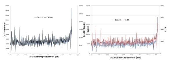
**Figure 8:** Ablation profiles on 5A2 along the yellow dotted track in figure 5. Left, overlaid Cs-133 & Ce-140 profiles. Right, overlaid Cs-133 & I-129 profiles (10 µm beam).
