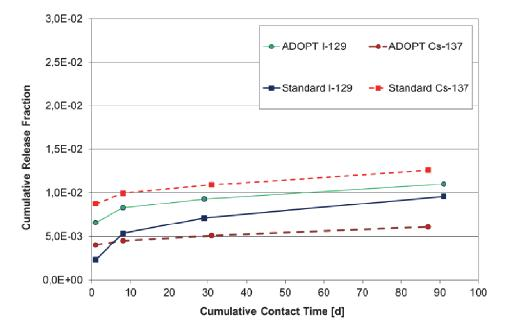
Figure 3: <sup>137</sup>Cs and <sup>129</sup>I cumulative release fractions from standard and Al/Cr doped fuel.
