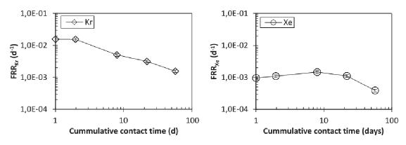
Figure 4: Fractional release rate of Kr (left side) and Xe (right side) as function of the cumulative contact time.
