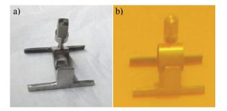
Figure 2: a) sample holder used during the experiment; b) sample holder mounted with pellet before immersion into the solution.
