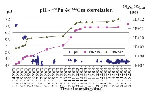
Figure 2: Change of pH and <sup>238</sup>Pu and <sup>242</sup>Cm activity concentration.
