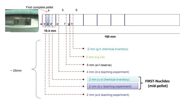
*Figure 5: BWR54* cutting plan showing the position and the nominal length of samples cut mid-pellet for IRF leaching studies and for further characterisations (solid vertical lines indicate pellet-pellet gaps; dashed lines indicate cut positions).
