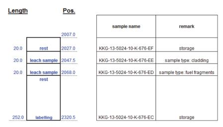
Figure 5: Segment cutting plan of the selected MOXPWR fuel.
