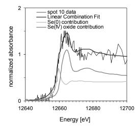
*Figure 5*: *Example of a LCF of the Se K-edge XANES data from Se(0) and Se(IV) reference compounds for an individual Se K-edge XANES spectrum collected on the spent fuel sample (spot 10).*
