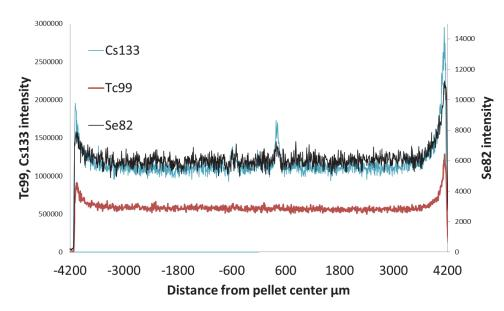
Figure 14: Ablation profiles on sample C1 (60 µm beam).
