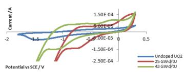
**Figure 4:** Cyclic Voltammogram of Undoped  $UO_2$ , 25 GWd/t<sub>U</sub> and 43 GWd/tU SIMFUEIs in modified simplified Groundwater, sparged with Argon.
