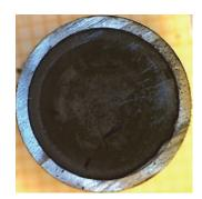
Figure 2: Cross section of the selected cladded fuel sample.
