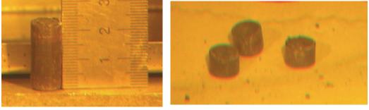
Sample of SNF for leaching test 1 The three pieces (0.8 cm each) of the sample prepared for leaching test 2 'Decladded sample'
