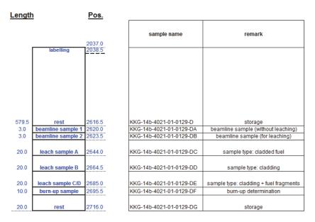
Figure 3: Segment cutting plan of the selected UO<sub>2</sub> PWR fuel.
