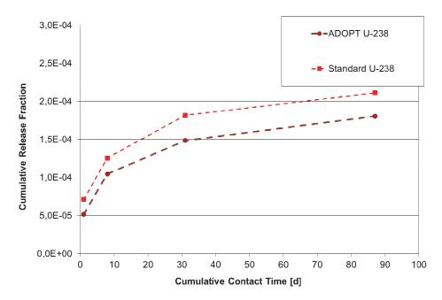
Figure 4: <sup>238</sup>U cumulative release fractions from standard and Al/Cr doped fuel.
