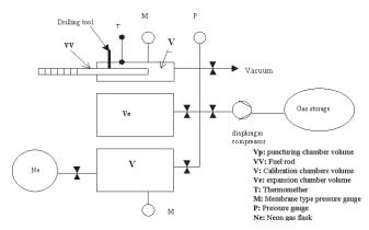
Figure 1: Scheme of the puncturing device (from Wegen et al., 2012a).
