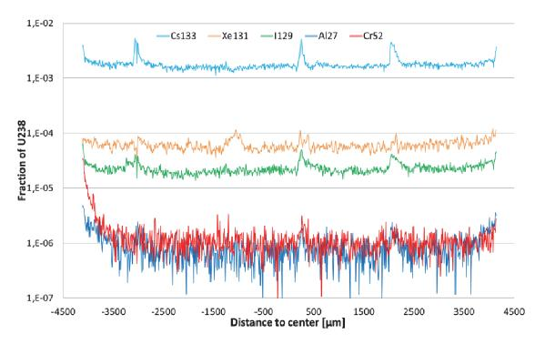
Figure 7: Ablation profiles on 5A2 along the green track in figure 5 (60 µm beam).
