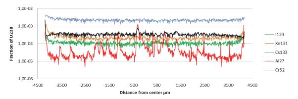
Figure 10: Ablation profiles on sample C1 along the track marked 1 in Figure 9 (60 µm beam).
