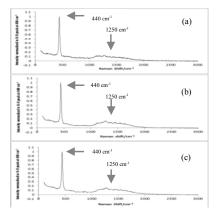
**Figure 1:** Micro-Raman spectra of an undoped  $UO_2$  sample: (a) as received; and after 1 h exposure to (b) oxygenated water and (c) 100  $\mu$ mol/dm<sup>3</sup> H<sub>2</sub>O<sub>2</sub>
