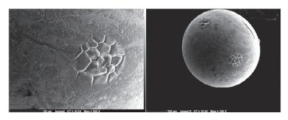
Figure 2: SEM pictures of the surface of a UO<sub>2</sub> particle corroded in open air atmosphere.
