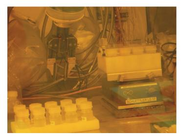
Figure 3: Experimental set-up (orbital stirrer).
