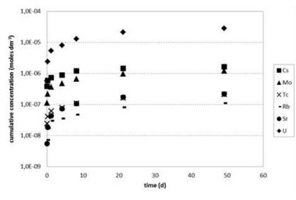
Figure 6: Elemental cumulative concentration (moles/dm) vs time.
