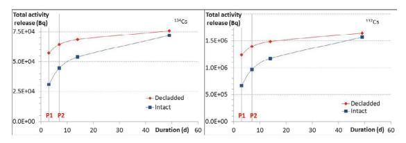
*Figure 3:* Evolution of the activity of <sup>134</sup>Cs (left side) and <sup>137</sup>Cs (right side) for the test with the "intact" and "decladded" fuel. P1 and P2 correspond to the two renewals of the solution during the preleaching steps.
