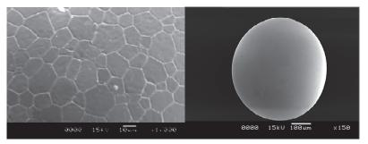
Figure 1: SEM picture of the surface of an unirradiated UO<sub>2</sub> particle.
