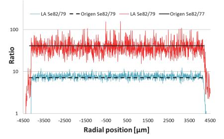
Figure 16: Comparison of Se isotope ratios from LA and average values calculated by the Origen code, sample C1 (60 µm beam).
