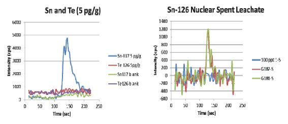
Figure 9:. (A) Behaviour of Sn and Te in the chelating column. (B) Detection of <sup>126</sup>Sn in nuclear spent fuel leachates (dilution 1/10).
