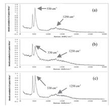
Figure 3: Micro-Raman spectra of a 43 GWd/tU SIMFUEL sample: (a) as received; and after 1 h exposure to (b) oxygenated water and (c) 100  $\mu$ mol/dm<sup>3</sup> H<sub>2</sub>O<sub>2</sub>
