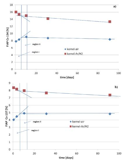
Figure 4: FIAP values for a) <sup>134</sup>Cs (%) and b) <sup>137</sup>Cs (%) under oxic and anoxic/reducing conditions.
