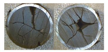
Figure 1: Two-face macroscopic view of the selected SNF cladded piece.
