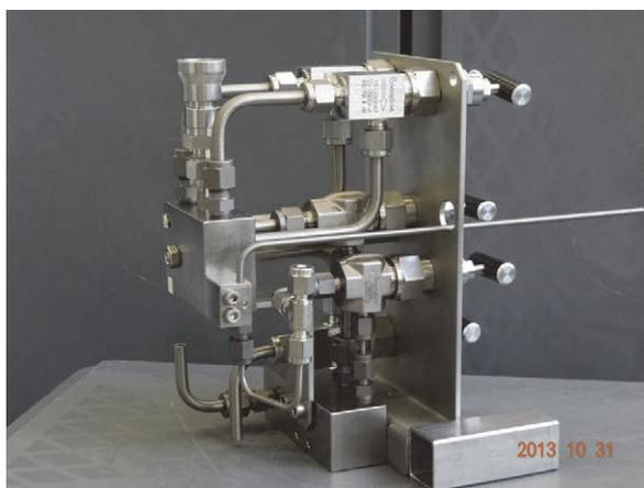
**Figure 2:** Manufactured autoclave head.
