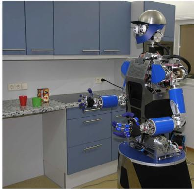
Figure 1.3.: Humanoid robot ARMAR-III, developed for applications in human-centered environments like service tasks in a household scenario (from [ARA<sup>+</sup>06])
