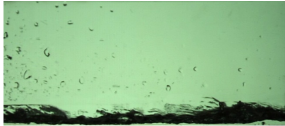
MP: 23 \dot{V}_{\text{Luft}} = 160 \text{ l/s} \dot{V}_{\text{Wasser}} = 55 \text{ l/min}
